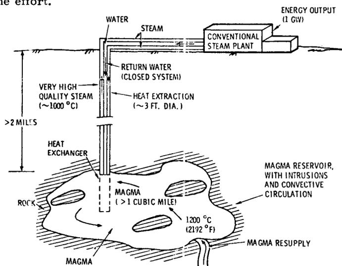
Figure 1. Generalized drawing of the magma tap concept
