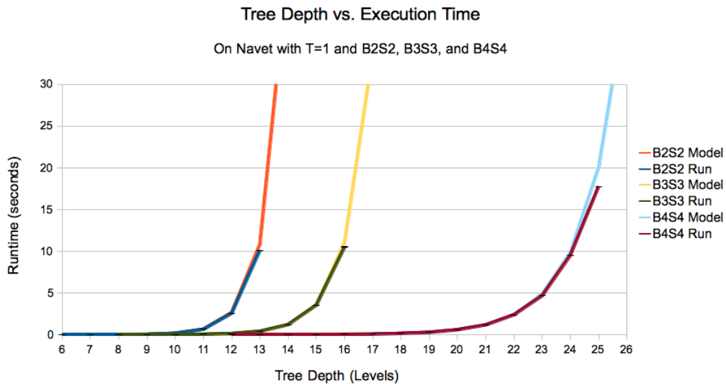
Figure 4.5. The effect of D on query execution time on Navet. Comparison of test results to performance model estimates for three different tree shapes.
