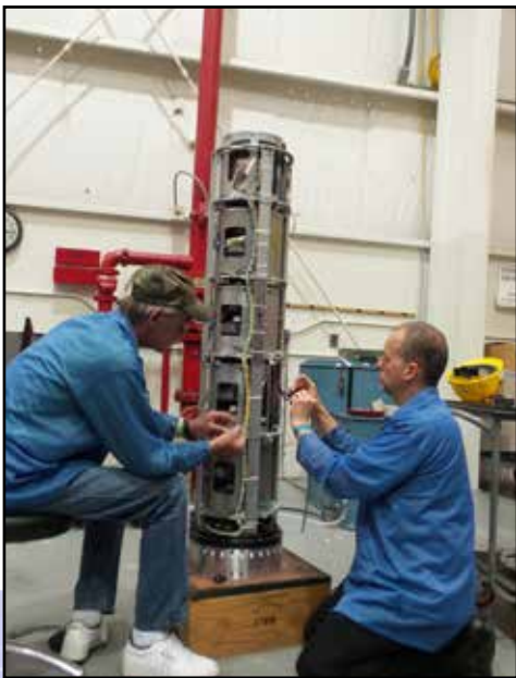
NASA staff integrating all participant payloads into the rocket.
