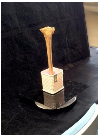
Figure 4.8. Set up of bone in shallow container.
