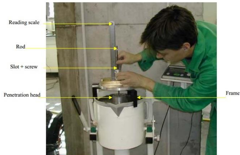
Figure 2-5 Penetration apparatus (De Schutter, 2005)
