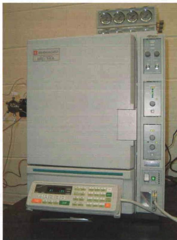
Figure A.6. Photograph of the Shimadzu Model 14A gas chromatography.
