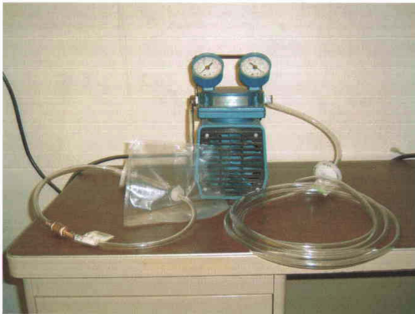
Figure A.4. Photograph of the gas sampling system.
