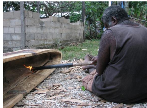
Apia experiments with a water sealant by melting PVC and pouring it into gaps in the hull.
