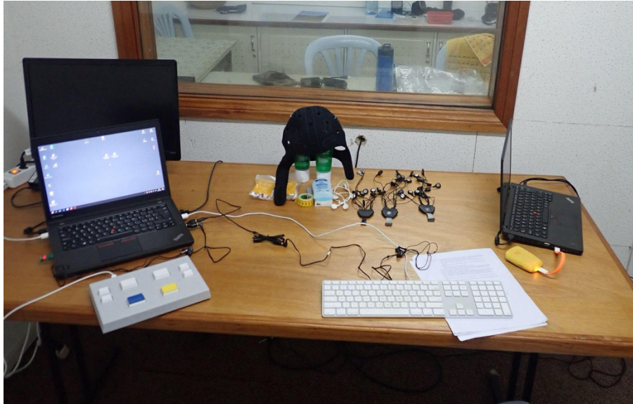
Figure 1. Exposition of the setup for EEG sentence comprehension experiment in Äiwoo. On the left, the “display” computer (which presented visual cues throughout the experiment, played back the audio stimuli, and recorded button press responses) with the button box can be seen. On the right, the recording computer is positioned so that the experimenter can monitor the EEG signal’s quality while remaining out of the immediate field of view the participant. The Neuroelectronics Enobio 32 amplifier is being charged. In the middle, the elastic cap which holds the electrodes in position on the scalp, as well as the system’s three electrode strings are placed.
