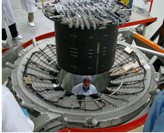
Figure 2.8 The assembled inner tracker being set inside the magnet.
