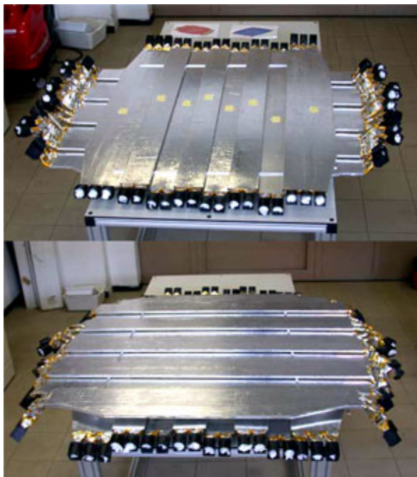
Figure 2.5 The upper and lower TOF planes that make the TOF system.
