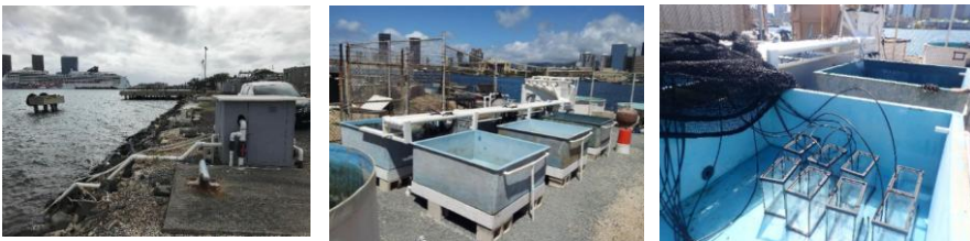
Figure 4. Facilities at AFRC Mesocosm use an Open Flow Sea Water System. From left to right; Pump house that takes in sea water from an 8 m depth. Mesocosm with PVC piping to distribute filtered sea water. Aquaria within mesocosm that housed plants during experiment.
