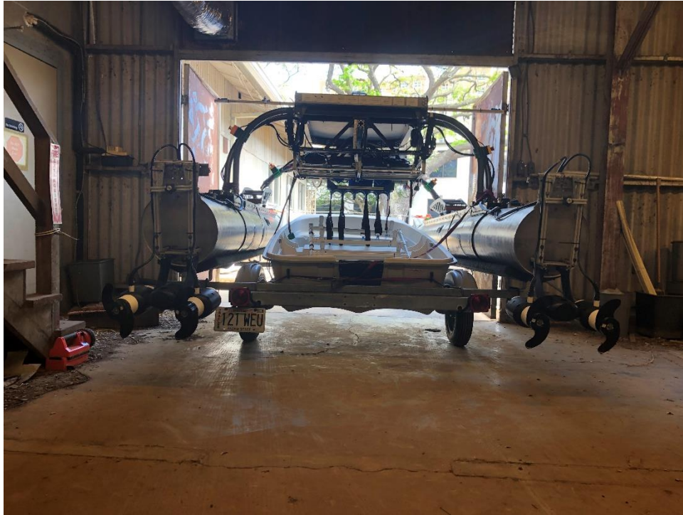
Figure 3: Rear view of WAMV with Minn Kota motors
