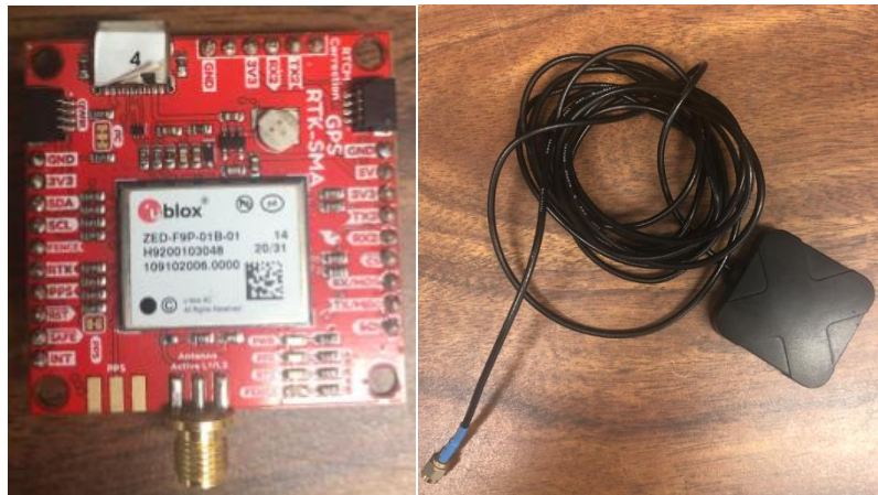
Figure 4: SparkFun ZED-F9P RTK GPS board (left) and Taoglas antenna (right)
