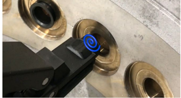
Figure 9: Detected collision, starting spiral search to find correct assembly position
