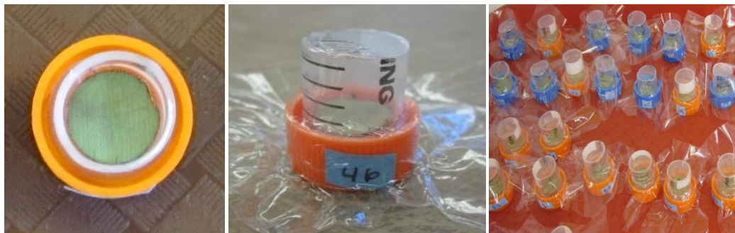
Plate IV. Cage used to observe individual aphids (belonging to a cohort) from birth until death for age specific molting, reproduction and survival during the life table study.
