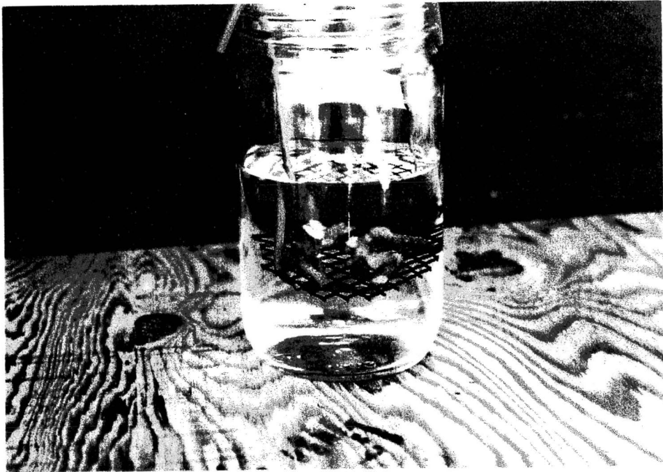
Figure 3. Bioassay container with polyethylene mesh platform and five coral branches.
