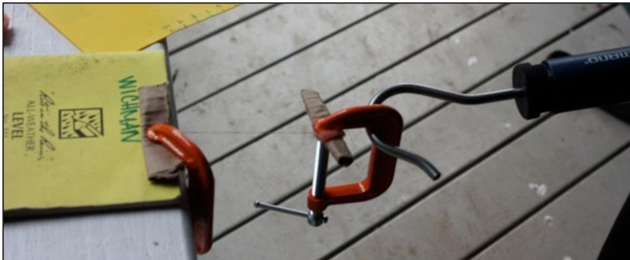
**Figure 3.** Experimental method for testing strength of *olonā* (*Touchardia latifolia* Gaudich.) cordage in Hā'ena, Kaua'i. Two C-clamps secure each end of the cord within a fold of cardboard. One end is secured to a fixed object (table) and the other to a scale used to measure the breaking strength.
