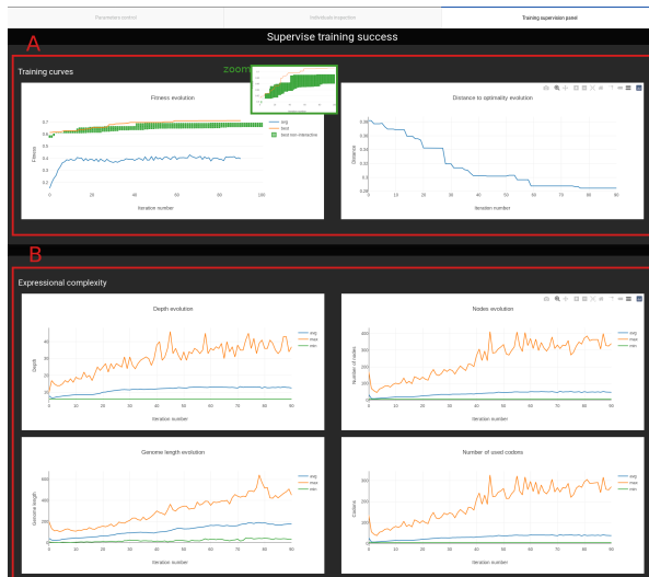
Figure 6. Training supervision tab. Zone A describes the scores evolutions while zone B give insights on the evolution of the population complexity.
