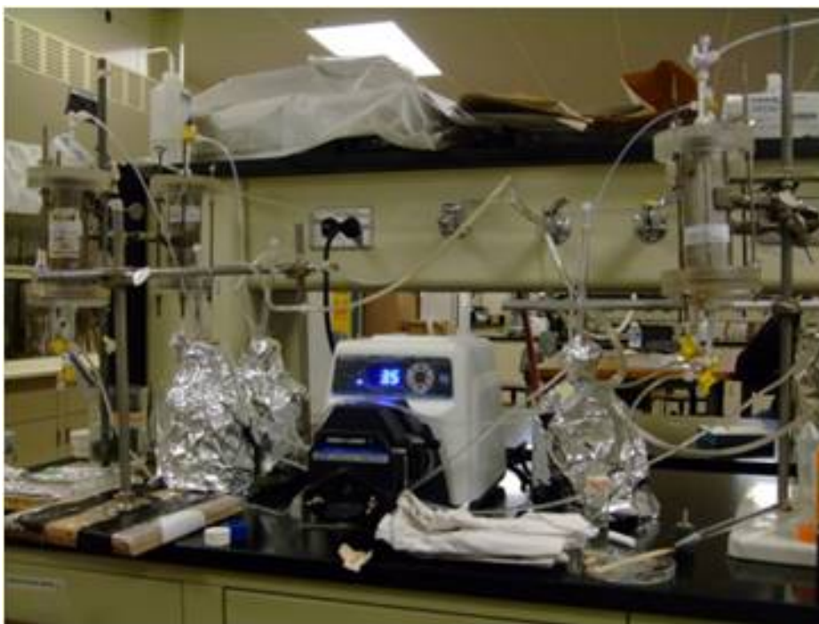
Fig. A4: Experimental set-up used in chapter 4 (column experiments conducted under re-circulated conditions).
