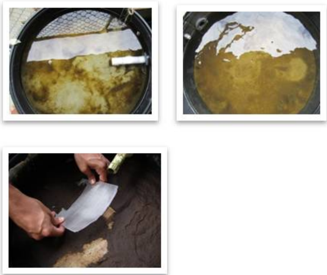
Fig. A3. Dynamics of the biolayer in a slow sand filtration (SSF) unit.
