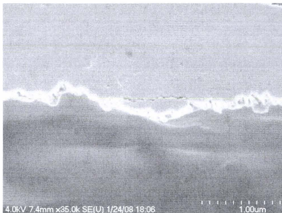
Figure 4.4. SEM cross-sectional view of platinum nanowires on Nafion® NRE-211 taken at a 45° stage tilt showing the aligned structure of the nanowires.
