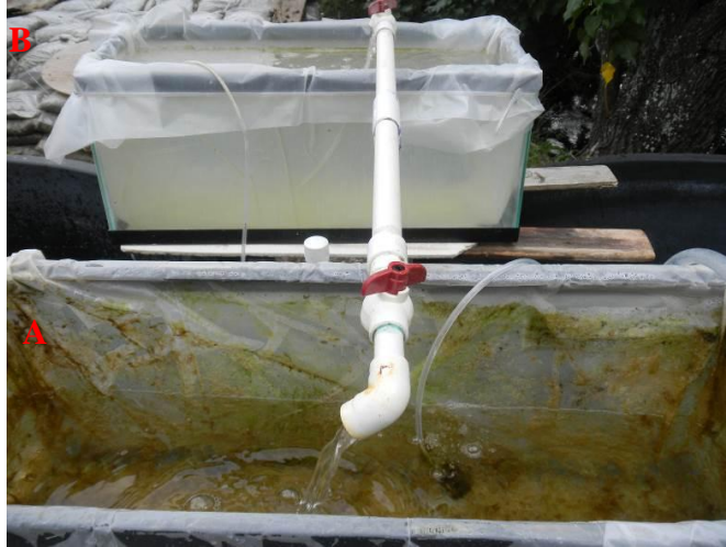
Figure 2.4. Diatom growth on rough plastic (A) and clear plastic (B) sheet at Day 7.
