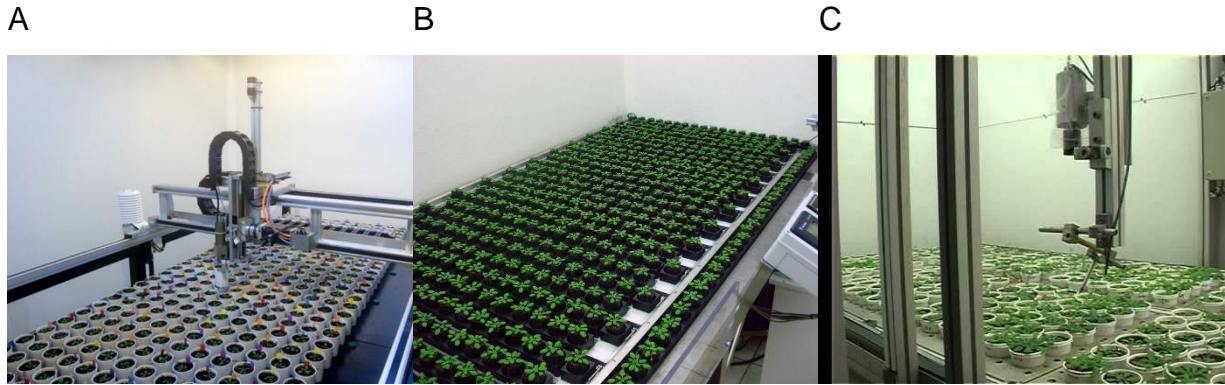
Figure 1.2. Examples of available automated phenotyping machines. Their nicknames are WIWAM (A), Phenoscope (B) and Phenopsis (C).
