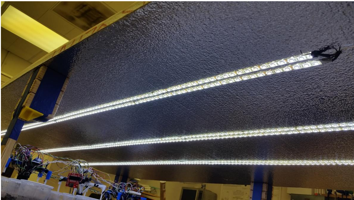
Figure 4.4. Styrofoam with LED lights attached.
