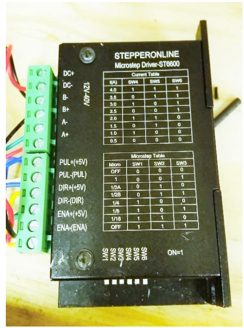
Figure 4.9. Stepper Motor Driver, ST-M5045 (Left) for Y-axis Stepper Motor and ST6600 (Right) for Z-axis Stepper Motors.
