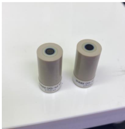
Figure 4.2 Two RRDE tips with identical specifications (left) with dried thin-film catalyst applied on the inner disk electrode (right) bare glassy carbon disk without added thin-film catalyst, for visual comparison.
