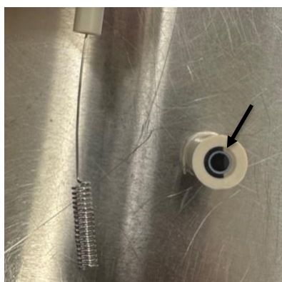
Figure 5.14 Photo of (left) Pt counter electrode vs (right) ring in RRDE tip (arrow pointing to outer ring electrode)
