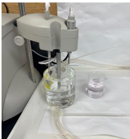
Figure 4.6 Example of the adjacent beaker with 0.1 M \text{H}_2\text{SO}_4 and 0.002 M \text{KMnO}_4 for visual comparison.
