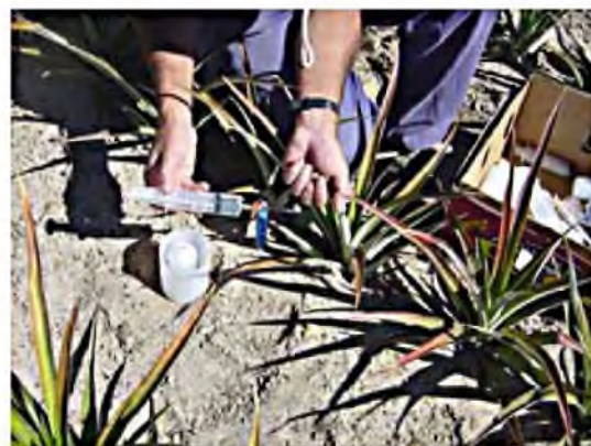
Field testing soil nitrogen levels using Mottet tubes.
