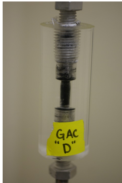
Figure 15: GAC Column During a Run
