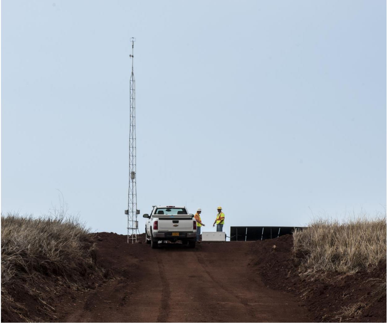
Figure 6 Photograph of instrument tower site 1 located on the upwind NE side of GPQ. It measures wind speed at 2m and 10m.
