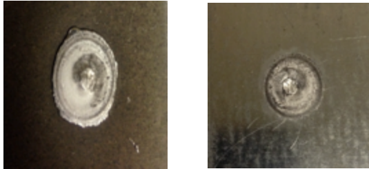
Fig. 3.8 Broken samples' result from the PIN failure. From left to right: upper plate viewed from the bottom, bottom plate viewed from the top
