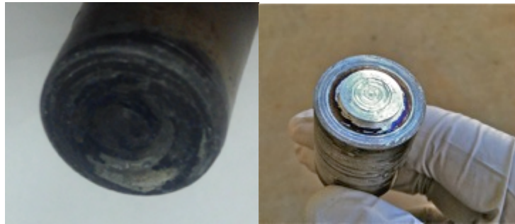
Figure 2.4, left: Si 3 N 4 tool, right: H13 steel tool
