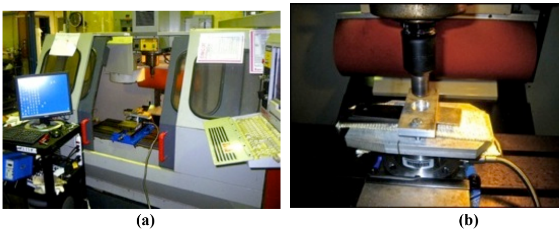
Fig. 2.5: Setup of CNC FSF experiments (a) Setup in CNC with measurement equipment (b) close up view of tool and fixture [sladjan, 2013]
