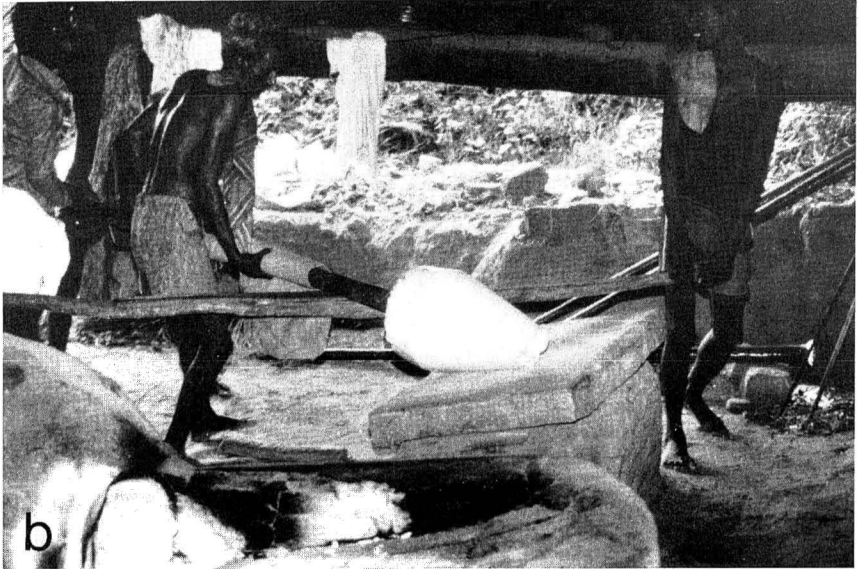
Pl. III. a . Glass on the gedda paru melting in the furnace. b . Once the glass is melted it is put on the lada and shaped into a cone. The trough for initial melting is visible in the foreground.
