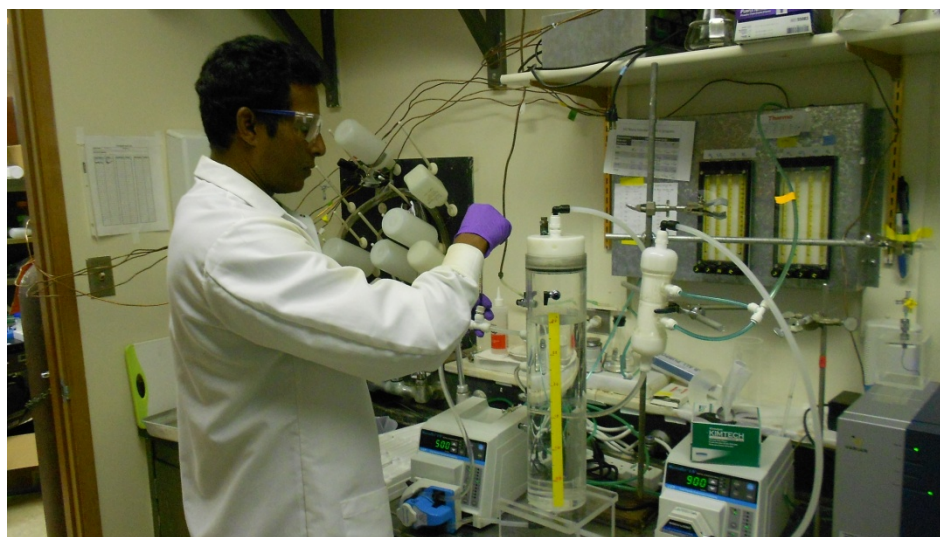
Figure A.4. Liquid sampling from the CHF membrane reactor
