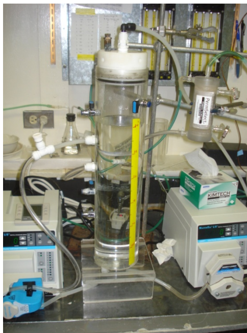
Figure A.5. Experimental set-up with PDMSXA-8300 membrane module
