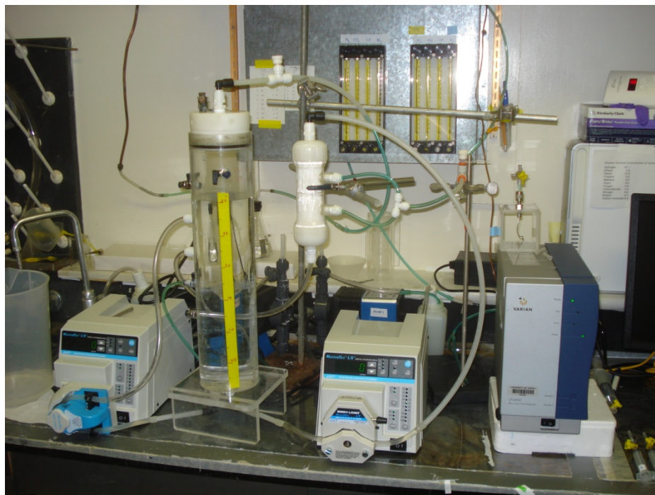
Figure A.3. Experimental set-up with composite hollow fiber (CHF) membrane module
