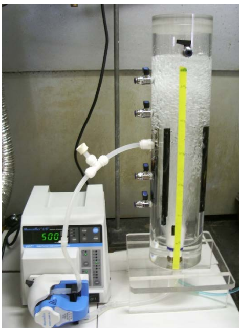
Figure A.2. Experimental set-up with gas-lift reactor combined with 20- \mu m bulb diffuser
