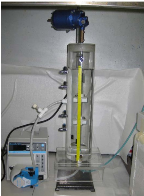
Figure A.1. Experimental set-up with mechanical mixing
