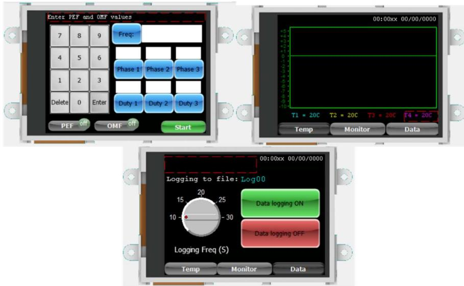
Figure 17. Selected UI interface pages created within the 4d-Workshop-4 IDE using the built in ViSi-Genie tool.
