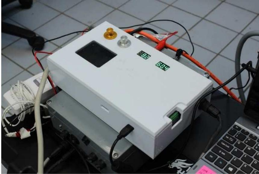
Figure 20. Control unit fully assembled. In the image above the unit is operating in USB data logging mode.
