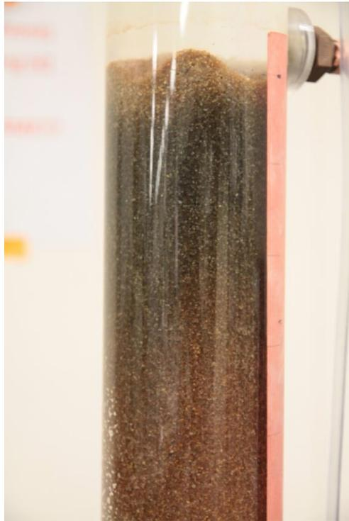
**Figure A.4. FeOOH coated sand column at initial time**
