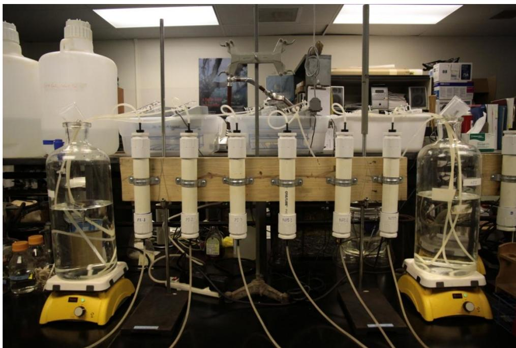
**Figure A.2. The microcosm MLS system**
