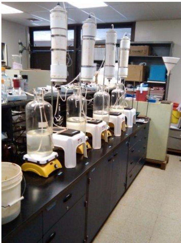
**Figure A.1. The Multi-Soil-Layer filter system**
