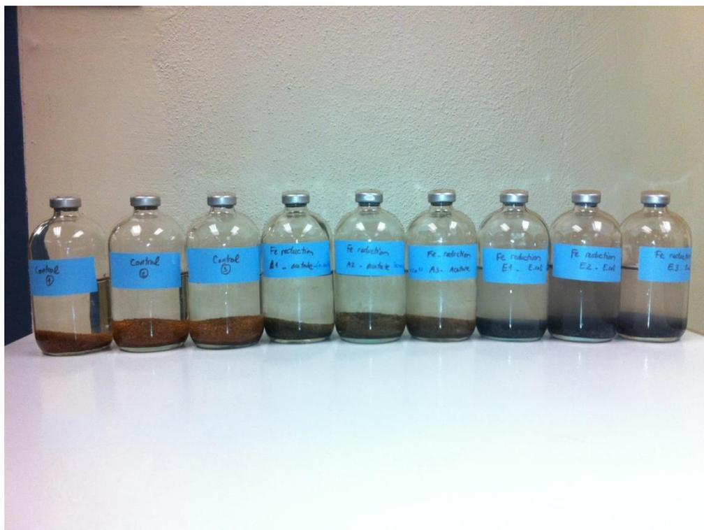
**Figure A.3. MIR microcosm setup for using *E. coli* as a source of electron donor**
