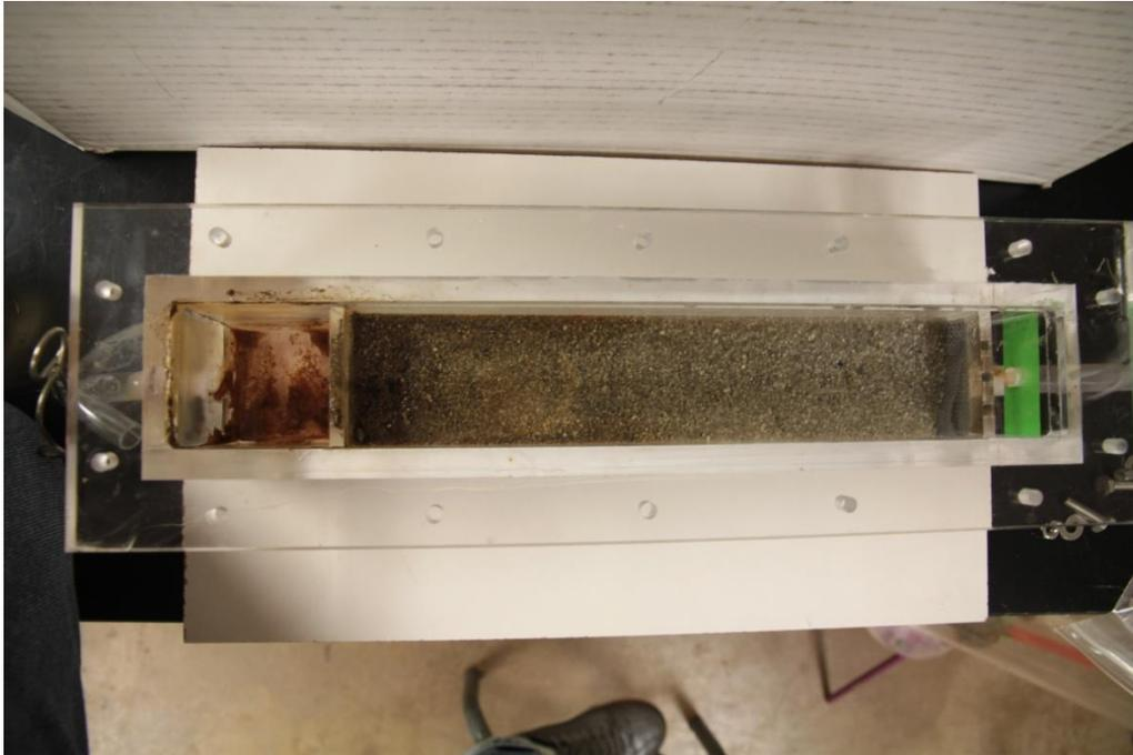
**Figure A.10. The horizontal aerobic filter**
