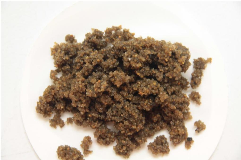
**Figure A.11. Precipitation of ferric oxides in the aerobic filter.**
