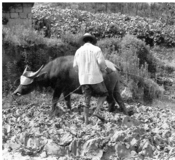
Figure 3.168. Blindfolded and led to walk in circles, this water buffalo is passing repeatedly over a mass of local river mud in order to work it into a suitable consistency for tile-making. Zhejiang. [RGK photograph 1987.]
