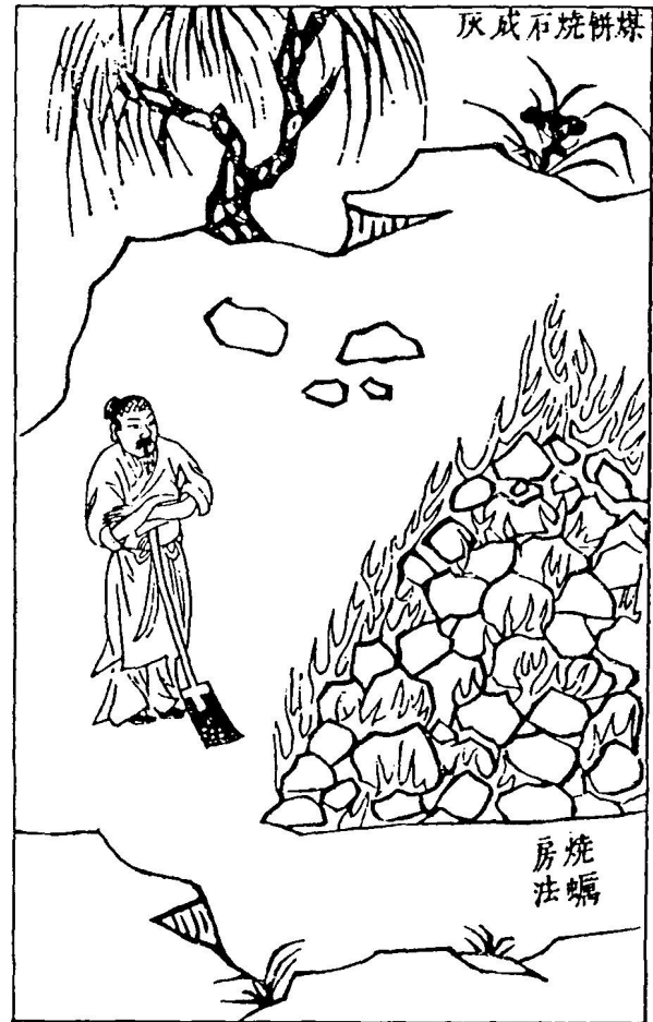
Figure 3.154. When mixed with other materials, lime is important as a water repellent and sealant. In villages all over China, the calcination of limestone or shells of oysters is an old practice that is necessary in house construction. [Source: Sung 1966, 200.]
