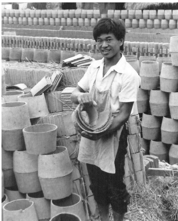
Figure 3.173 (top left). Once shaped, the now tubular clay sheet is carried on the mold to a drying area. There the wooden mold is collapsed, separating it and the moistened cloth from the tubular clay shape. The clay shapes are stacked to air dry. Zhejiang. [RGK photograph 1987.]
