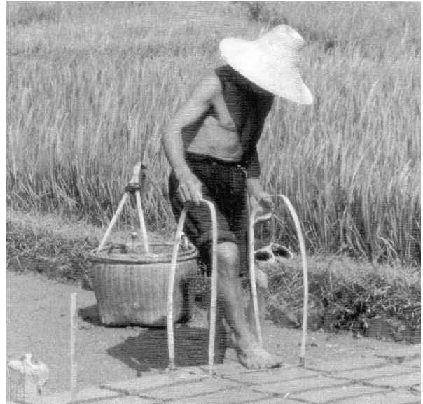
Figure 3.88. Bricks cut from paddy fields not only produce a necessary building material but provide a means to correct the natural siltation of fields. Baisha xiang, Lipu xian, Guangxi Zhuang Autonomous Region. [RGK photograph 1984.]
