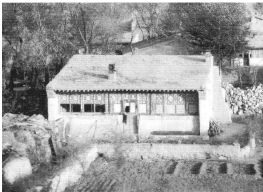
Figure 2.11. With lattice windows across its south-facing facade, this three- jian dwelling has an entry into the central room. The placement of only a single chimney indicates the presence of only one kang in the westernmost jian . Central Shanxi. [Original photograph courtesy of Arthur J. Van Alstyne.]
