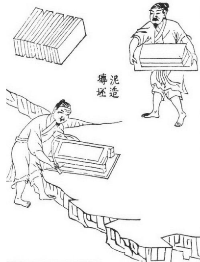
Figure 3.84. The seventeenth-century technical manual Tiangong kaiwu [The creations of nature and man] illustrates the use of wooden frames to mold bricks and a wire-strung bow to cut them evenly. [Source: Sung 1966, 139.]
