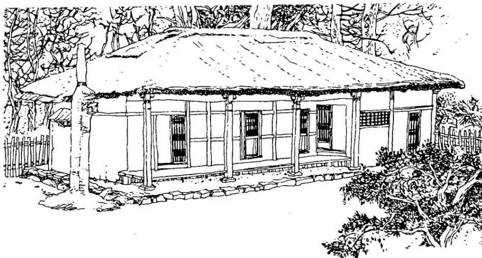
Figure 4.16. Appearing very much like dwellings in nearby areas of the Korean peninsula, this dwelling has an earthen/thatched roof with a colonnaded porch at the front. Along the side is a chimney made of wood and mud bricks that is set a meter or so from the dwelling. [Original drawing used with the permission of Wang Qijun. Source: Wang 1993, 71.]
