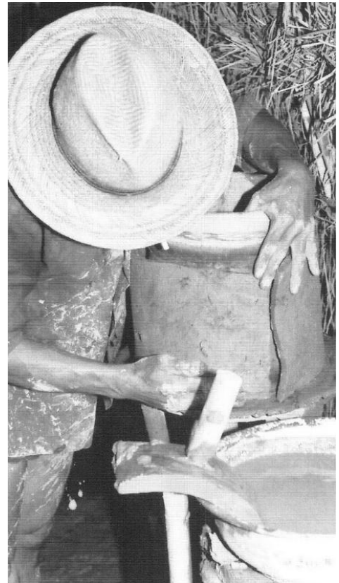
Figure 3.171 (top right). Initially the sheet of clay on the wooden mold is smoothed with the hands. A shaping tool and vat of water, which will be used later, are shown in the foreground. Zhejiang. [RGK photograph 1987.]
