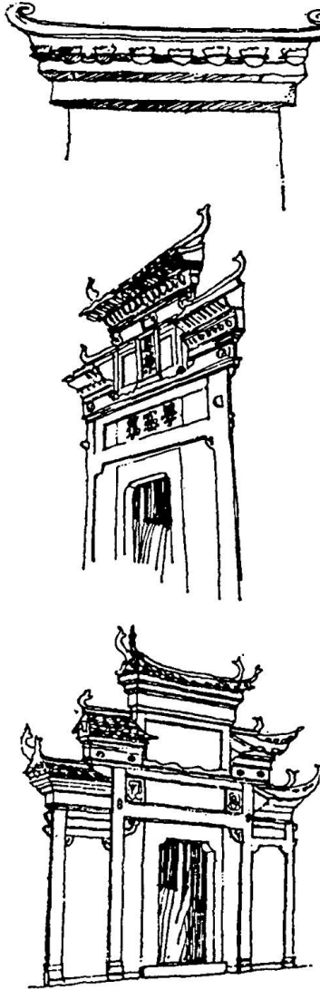
Figure 5.45 (above). The wealth and status of the head of a household can be inferred from the entryway, which may range from a simple menzhao or "canopy" covering (top) to a more complex menlou , a multi-level flat arch "structure" (bottom). [Source: Zhang et al., 1957, 18.]
