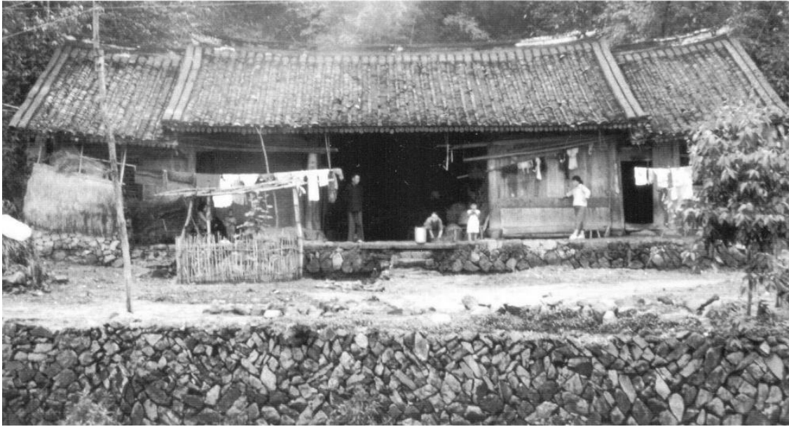
Figure 2.6 (above). This rectangular three-bay southern dwelling has two additional lower bays added to it. The central bay is somewhat wider than the adjacent ones and it lacks an exterior wall in the front, creating an “open room,” or changting , which will be discussed later. Shuitou xiang, Cangnan xian, Zhejiang. [RGK photograph 1988.]
