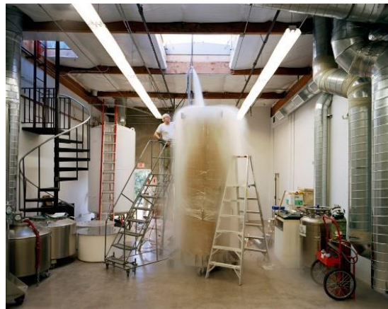
Figure 19. Dewar being filled with liquid nitrogen 25
