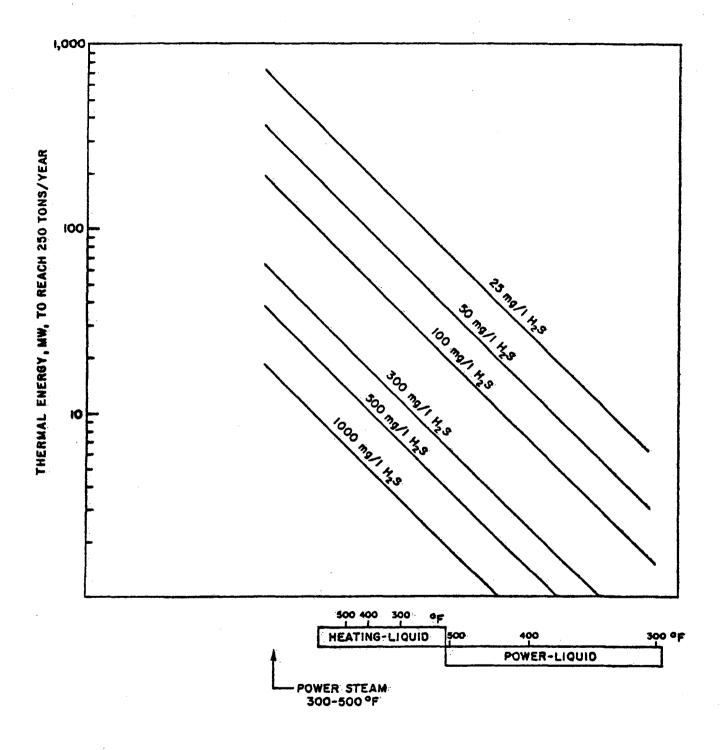
FIGURE 5. THERMAL ENERGY WHICH CAN BE PRODUCED WITH LESS THAN 250 TONS/YEAR HYDROGEN SULFIDE EMISSIONS, WITHOUT CONTROL EQUIPMENT
