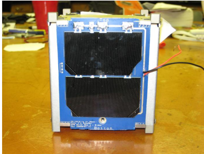
Figure 2: Populated Solar Panel on Engineering Model (EM)
