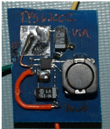
Figure 6: Prototyped TPS63002 Circuit
