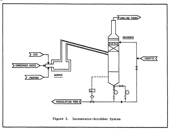
elemental sulfur formation downstream of the incinerator. Sulfur deposition in the scrubber column packing resulted in rapid plugging and a high pressure drop across the column. Modification of the air feed system to increase the air supply rate, to twice the stoichiometric air requirement, alleviated this problem for routine operations. However, occassional recurrance of "flame out" conditions in the incinerator tank continue to generate a gradual build-up of sulfur in the column packing.
