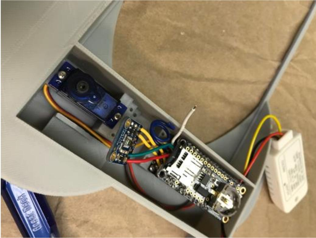
Figure A3: The Adalogger FeatherWing has been attached to the Feather M0.
