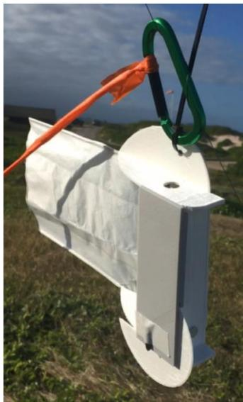
Figure 11: A photograph of a mini-GNI instrument attached with a carabiner to the kite string using a black zip tie. Notice that the door is closed until the instrument reaches the desired altitude, and an orange streamer is also attached for visibility.
