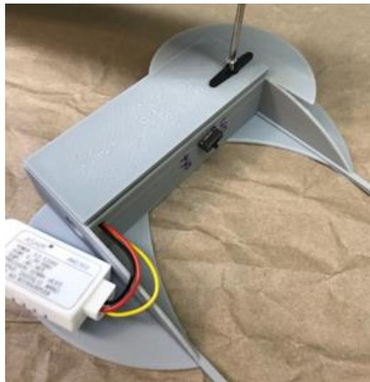
Figure A8: The door is screwed into place to the Micro Servo. The AM2302 sensor is attached to the side via adhesive putty as seen in Figure 5.
