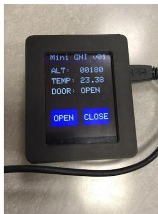
Figure 8: A photograph of the touchscreen control station used to communicate with the mini-GNI instrument from the ground while the mini-GNI is aerially deployed.
