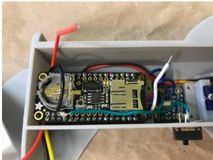
Figure A5: The SPDT slide switch used to power the instrument on and off has been put into place.
