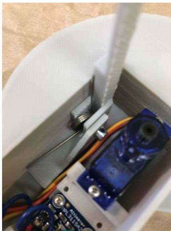
Figure A6: The arm is put in place with the spring, clevis, and cotter pin.
