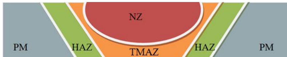
Figure 2: Typical cross section of FSW displaying the various zones.
