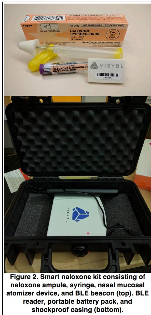
**Figure 2. Smart naloxone kit consisting of naloxone ampule, syringe, nasal mucosal atomizer device, and BLE beacon (top). BLE reader, portable battery pack, and shockproof casing (bottom).**
