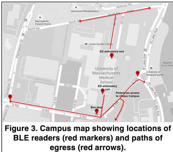
By selecting BLE readers with adequate range to cover major road intersections and power to penetrate cars, we can detect the transit of smart naloxone kits off of a hospital campus. This approach is highly scalable—rapid deployment of BLE readers throughout a community in response to an escalating heroin epidemic can help public health officials and researchers discover hotspots of naloxone as a marker
