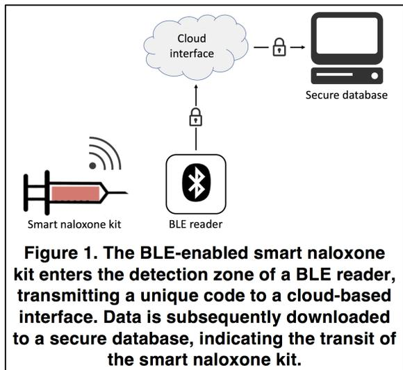
**Figure 1. The BLE-enabled smart naloxone kit enters the detection zone of a BLE reader, transmitting a unique code to a cloud-based interface. Data is subsequently downloaded to a secure database, indicating the transit of the smart naloxone kit.**
