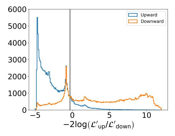
Figure 5.7: Log-likelihood confidence distribution of a random subset of about 230,000 of the simulated  $\alpha$  tracks described in Chapter 5.2. True upward pointing tracks are shown in blue and true downward pointing tracks are shown in orange. The black vertical line represents the chosen value of c for which all events to the right (left) of this line are assigned to be downward (upward) facing by the LL method.
