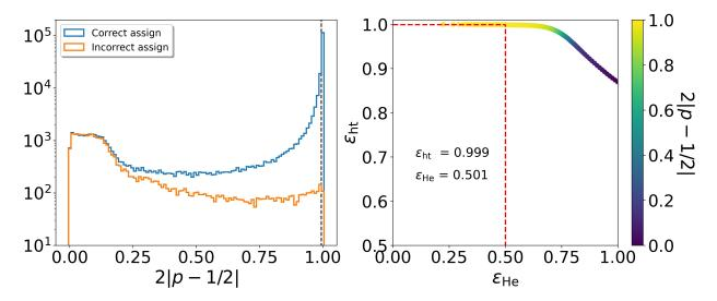
Figure 5.15: Left: Distribution of  $w = 2|p_- - 1/2|$  with correctly assigned events in blue and incorrectly assigned events in orange. The vertical black dashed line indicates the value above which we have  $\varepsilon_{\text{He}} = 0.5$ . Right: ROC curve showing  $\varepsilon_{\text{ht}}$  versus  $\varepsilon_{\text{He}}$  at various w selections. The 3DCNN is a nearly perfect classifier for this sample of events at 50% He recoil efficiency.
