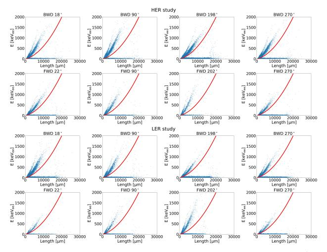
Figure 3.5: Energy versus length distributions of all tracks in each TPC during the HER (top two rows) and LER (bottom two rows) background studies. The red line in each plot shows our selection boundary; we keep all events with energies above this boundary.
