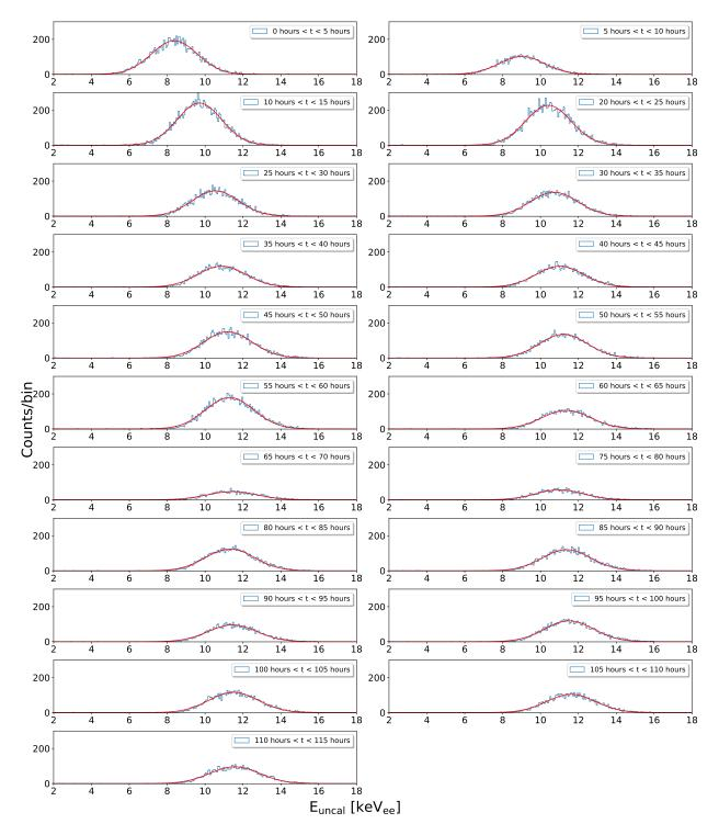
Figure B.2: Uncalibrated X-ray energy spectra at various time slices. The red curve shows a Gaussian profile fit with linear background to each distribution. The spectra shifting to the right over time is an indication of the gain increasing due to increasing He: $CO_2$  gas purity.
