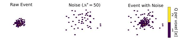
Figure 8.7: Comparison of raw event, a random noise distribution, and the "noisy event" when  $\mathcal{N}' = 50$ . Left: Raw 3D event display using the  $(850 \times 850 \times 850)\mu m^3$  segmentation. Middle: Random 3D noise distribution computed on a  $32 \times 32 \times 32$  grid with the same segmentation. Right: The combined "noisy event" containing all points from the raw charge distribution as well as the noise distribution.
