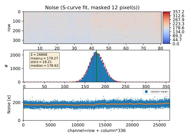
Figure 7.2: Same as Figure 7.1 but for noise distribution. The mean noise is about 30% of the mean threshold leading to a large uncertainty in threshold due to noise.
