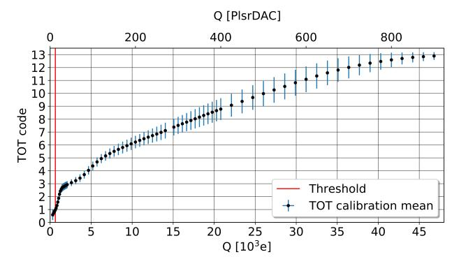
Figure 7.3: Average TOT response to 100 charge injections in all pixels over 70 distinct charge steps (charge steps are represented by points). The vertical red line shows our threshold which is what we set TOT = 0 to be.
