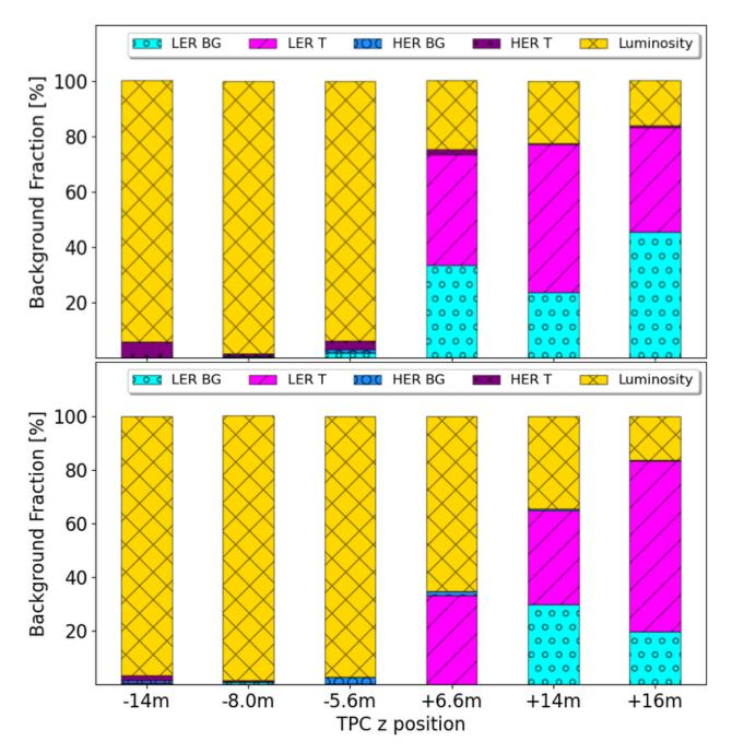
Figure 4.8: (color online) Background compositions determined from fits to storage fills extrapolated to the machine parameters shown in Table 4.4 for Study A (top) and Study B (bottom).
