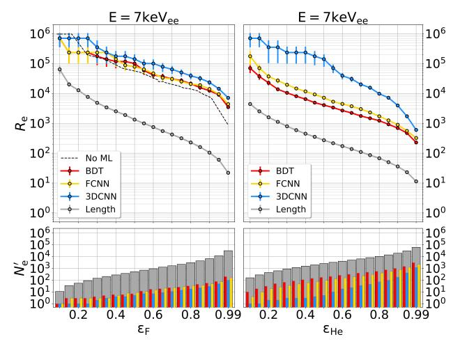
Figure 8.5: Comparison of electron rejection performance of all discriminants versus nuclear recoil efficiency for  $7 \text{ keV}_{ee}$  fluorine recoils (left) and  $7 \text{ keV}_{ee}$  helium recoils (right). The top and bottom row plots share a common horizontal axis. The black dashed line in the upper left hand plot shows the combined observable from Ref. [97]. The bottom bar plots show the number of remaining electrons after a given recoil selection in each efficiency bin.
