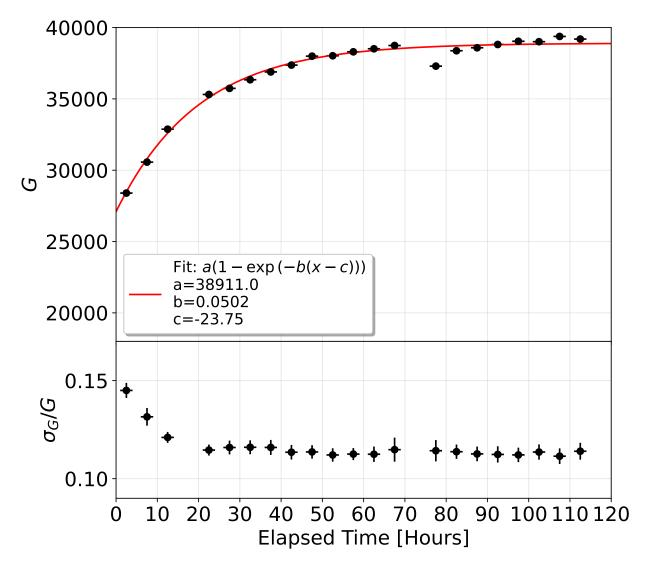
Figure B.3: Top: Gain determined by scaling the profile fits from Equation (B.3) to 5.9 keV versus time. Bottom: Gain resolution determined from the profile fits of Equation (B.3) versus time.
