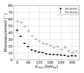
Figure 4.11: Mean (data points) and standard error (vertical error bars) of angular mismeasurement between SVD fits to the principal axis of the reconstructed simulated track and the truth MC-simulated direction of the recoil split up between <sup>4</sup>He recoils (filled points) and <sup>12</sup>C/<sup>16</sup>O recoils (unfilled points). The angular resolution of <sup>4</sup>He recoils is considerably better than <sup>12</sup>C and <sup>16</sup>O recoils.
