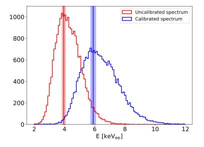
Figure 7.7: Uncalibrated (red) and calibrated (blue) energy spectrum of the  ${}^{55}$ Fe X-rays. The pale red and blue vertical bands show the uncertainty in the peak location.
