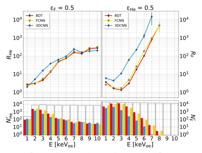
Figure 8.6: Comparison of He and F recoil rejection at fixed F and He signal efficiencies.  $R_{\text{He}}$  and  $R_{\text{F}}$  are rejection factors for He and F recoils, respectively and are both defined analogously to  $R_{\text{e}}$ . The bins in the upper right plot with no data points plotted have all F recoils rejected.
