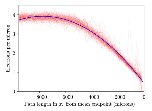
Figure 5.3: Taken from [82]: Simulated Bragg curves for one hundred 1 MeV alpha tracks (red lines) simulated in SRIM. Here positive  $x_t$  corresponds to the initial momentum direction of the recoil track with  $x_t = 0$  being the track's stopping end (head). The blue curve is a fit representing the average behavior of these Bragg curves. The negatively sloped region of the blue curve is what we refer to as the region beyond the Bragg peak.
