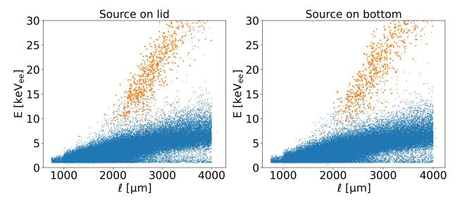
Figure 7.19: Selected signal sample of nuclear recoil candidates (orange) overlaid on top of all measured events (blue).
