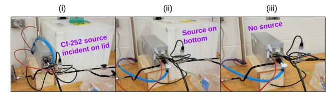
Figure 6.1: Lab set-up for low gain head-tail studies. We use a <sup>252</sup>Cf spontaneous fission source to generate neutron recoils for the TPCs. We record around one week of data both for the source-on-lid sample and source-on-bottom sample, and about two weeks of background "no source" data.
