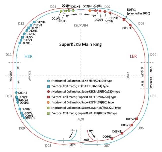
Figure 2.2: [38] The SuperKEKB collimation system is one of the primary means to mitigate beam backgrounds. The system contains 31 collimators at various points along the LER and HER. During the upgrade from KEKB to SuperKEKB, new collimators were installed both throughout the LER and along both rings near the interaction region (IR).
