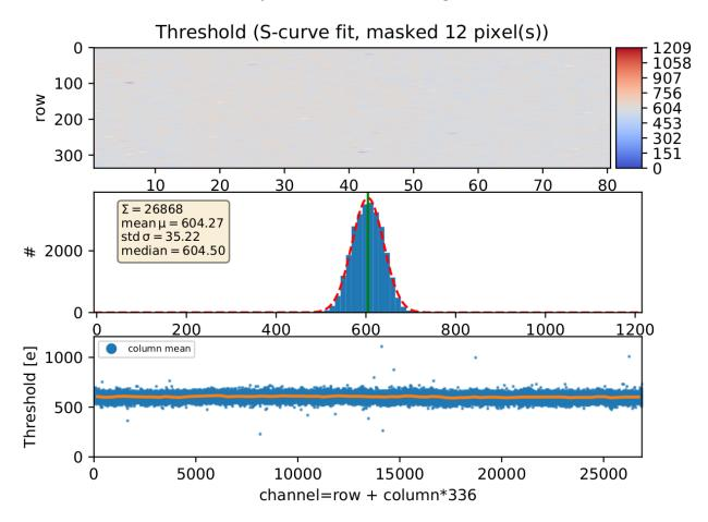
Figure 7.1: Top: Row versus column of the FE-I4 pixel grid with the color scale showing the threshold of each pixel. Middle: Threshold charge distribution with a fitted Gaussian profile. The variance in threshold is in general low. Bottom: Threshold distribution plotted versus 1D pixel number.
