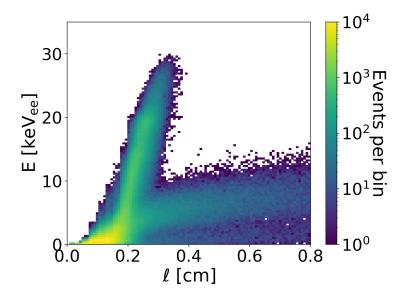
Figure 7.9: Reconstructed energy versus length of all simulated recoils in the high-gain campaign.
