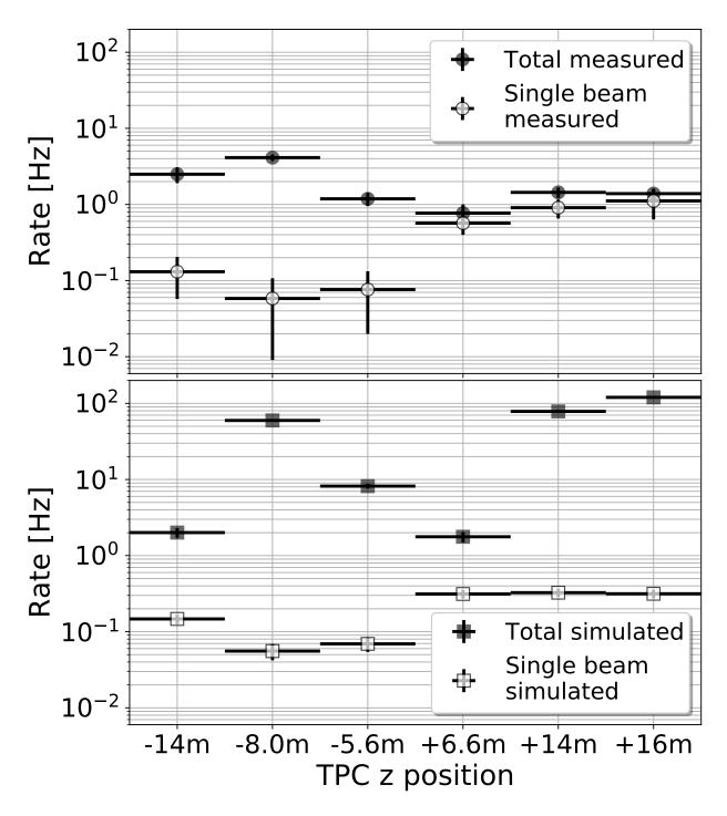
Figure 4.9: Comparison of single beam and total (single beam + luminosity) nuclear recoil rates extrapolated to the machine conditions listed in Table 4.4 for observed recoils during the luminosity decay fill periods of Study A (top) and simulated recoils (bottom).
