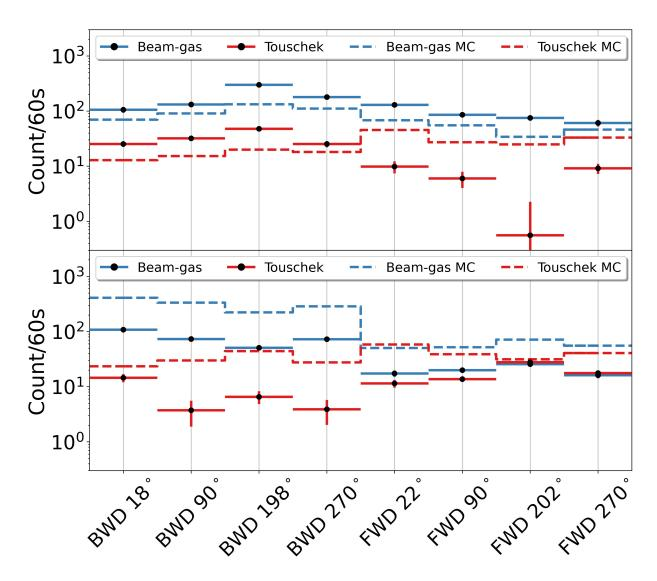
Figure 3.10: Comparison of modeled and measured beam-gas and Touschek backgrounds for the HER study (top) and LER study (bottom) in each TPC (TPC location listed as the horizontal axis label). The black markers with solid red and blue errorbars show measured rates and the dashed lines show simulated rates.
