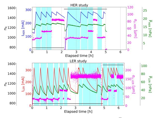
Figure 3.7: Beam currents, I, average beam-pipe pressures around the ring,  $\overline{P}$ , vertical beam sizes,  $\sigma_y$ , and numbers of bunches  $n_b$  plotted as a function of time over the course of the HER (top) and LER (bottom) studies. The cyan-filled regions represent beam storage periods where data was analyzed. We note that the largest HER beamsize periods are omitted from our analysis, due to an increase in background that wasn't understood at the time.
