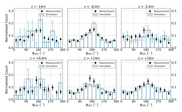
Figure 4.19: (color online) Comparison of  $\phi_{\text{TPC}}$  between measurement (black points) and simulated luminosity background nuclear recoils (blue bars) for events satisfying  $E_{\text{ionization}} > 40 \text{ keV}_{\text{ee}}$  during the luminosity decay fills of Study A. Histograms are constructed after applying final directional head-tail assignments.
