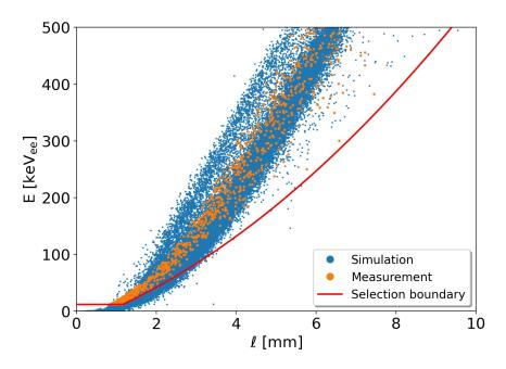
Figure 6.4: Energy versus length along principal axis distributions of measured and simulated tracks. Both measurement and simulation assume a gain of 910. Simulated tracks include only truth He recoils.
