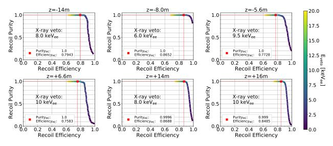
Figure 4.4: Simulated ROC curves showing nuclear recoil signal purity versus efficiency as a function of X-ray veto threshold energy for Study A. The boxes show the predicted nuclear recoil purity and efficiencies corresponding to the X-ray veto threshold decided for each TPC. Our procedure prioritizes selecting a veto with higher nuclear recoil purities than the X-ray veto threshold point that maximizes the area under the ROC curve.
