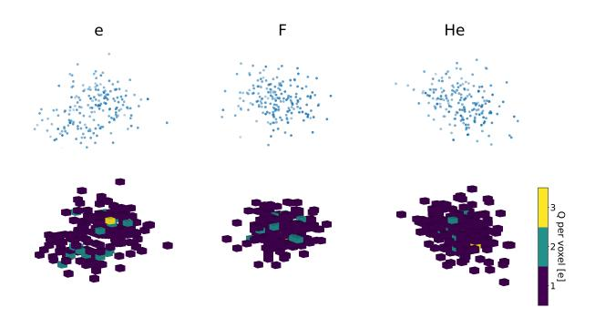
Figure 8.1: 3D charge distributions of  $6 \text{ keV}_{ee}$  electron, fluorine, and helium recoils after diffusion. The top row shows the original ( $100 \text{ µm} \times 100 \text{ µm} \times 100 \text{ µm}$ ) binning of these events, which is fine enough that there is only a single charge in each filled bin. The bottom row shows the events re-binned into the ( $32 \times 32 \times 32$ ) voxel grid that are input into the 3DCNN.
