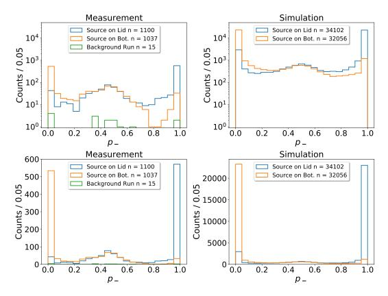
Figure 6.5: 3DCNN head-tail assignment for measured (left) and simulated (right) recoils. Individually the source-on-lid and source-on-bottom samples have strongly asymmetric  $p_{-}$  distributions in both measurement and simulation with the probabilities peaking in the expected direction of recoils coming from the source.
