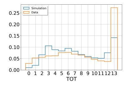
Figure 7.21: Comparison of charge (TOT) distributions of measured and simulated events satisfying  $2.0 \text{ cm} < \ell < 2.2 \text{ cm}$ . Both histograms are normalized to an integral of unity.
