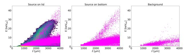
Figure 7.18: Observed recoil energy versus length distributions in each of the three measurement campaigns (magenta). The leftmost panel also shows a 2D histogram of simulated recoils with a logarithmic colorscale to highlight the agreement in dE/dx between measurement and simulation.
