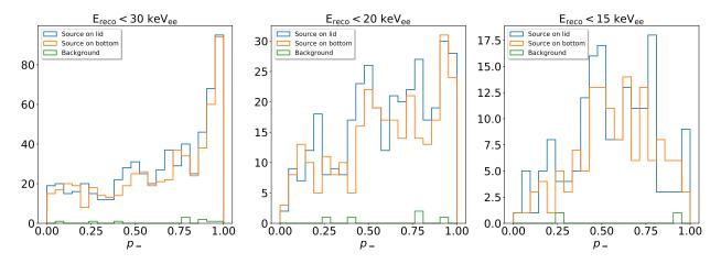
Figure 7.20: Distribution of output probabilities that the events lie in the negative  $\phi_{\text{truth}}$  hemisphere  $(p_{-})$ . We find little difference in the source-on-lid and source-on-bottom samples indicating that our trained 3DCNN does not provide meaningful head-tail assignment performance on measurement.
