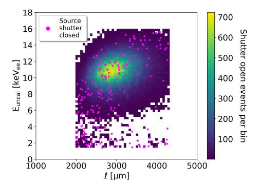
Figure B.1: Uncalibrated energy versus track length distribution of fiducialized events near the expected X-ray energy spectrum peak from the <sup>55</sup>Fe source. The 2D histogram shows events recorded when the source shutter was open and the magenta points show events recorded over the same amount of elapsed time with the source shutter closed.
