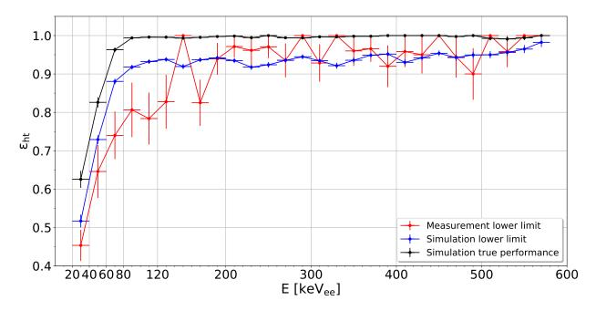
Figure 6.10: "Grand summary" comparison of head-tail assignment performance versus energy. Energy bins have width  $20 \text{ keV}_{ee}$  and for the events within each energy bin, we make selections on w corresponding to 50% He recoil efficiency and compute the head-tail recognition efficiency.
