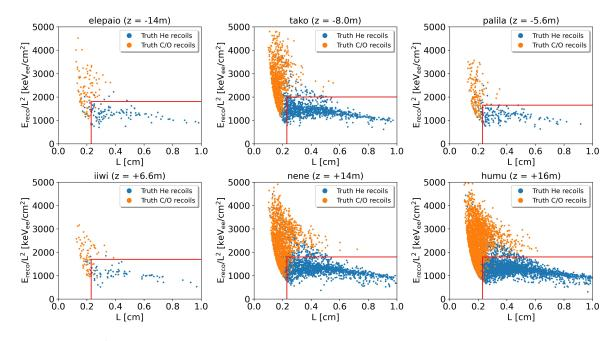
Figure 4.12:  $E/\ell^2$  versus  $\ell$  with truth simulated He recoils in blue and truth simulated C/O recoils in orange. Events within the red rectangle in the lower right hand corner of each plot are selected as He recoils.
