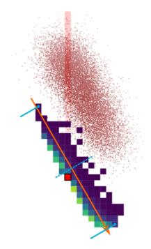
Figure 5.5: Taken from [82]: Illustration of head-tail mismeasurement resulting from the charge integration of a downgoing 400 keV<sub>r</sub> recoil with  $\theta_{\rm TPC} = 150^{\circ}$ .
