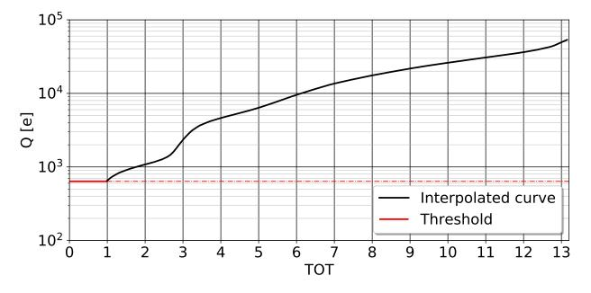
Figure 7.4: Bicubic spline interpolation over the points shown in Figure 7.3 shown as a black line. The charges where the interpolated curve matches an integer TOT code are what we set as the calibrated charge for a given integer TOT code.
