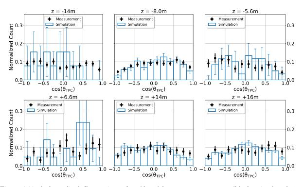
Figure 4.20: (color online) Comparison of  $\cos(\theta_{\rm TPC})$  between measurement (black points) and simulated luminosity background nuclear recoils (blue bars) for events satisfying  $E_{\rm ionization} > 40 \,\rm keV_{ee}$  and  $90^{\circ} < \phi_{\rm TPC} < 270^{\circ}$  during the luminosity decay fills of Study A. Histograms are constructed after applying final directional head-tail assignments.
