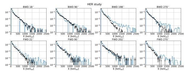
Figure 3.11: Comparison of measured (black points) and simulated (blue bars) nuclear recoil energy spectra above  $40 \text{ keV}_{ee}$  for the HER background study. All distributions have been normalized to an integral of unity.
