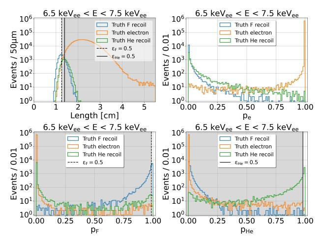
Figure 8.3: Comparison of traditional (track length) and 3DCNN-based ( $p_e$ ,  $p_F$  and  $p_{He}$ ) discriminants for events in the test sample satisfying 6.5 keV<sub>ee</sub>  $< E_{\text{ionization}} < 7.5 \text{ keV}_{ee}$ . The shaded regions in the panels indicate events that are rejected after selections corresponding to 50% F recoil efficiency (dashed black vertical line) and/or 50% He recoil efficiency (solid black vertical line).
