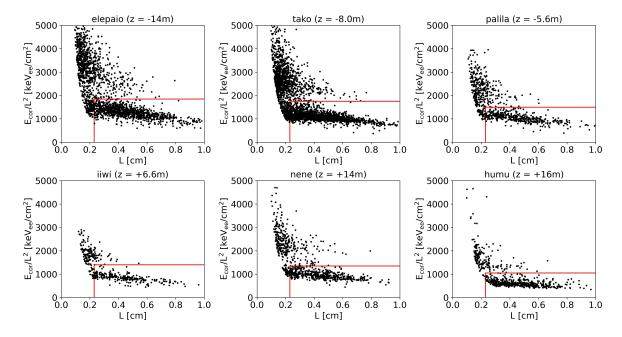
Figure 4.13: Measured  $E/\ell^2$  versus  $\ell$ . Events within the red rectangle in the lower right hand corner of each plot are selected as He recoils.
