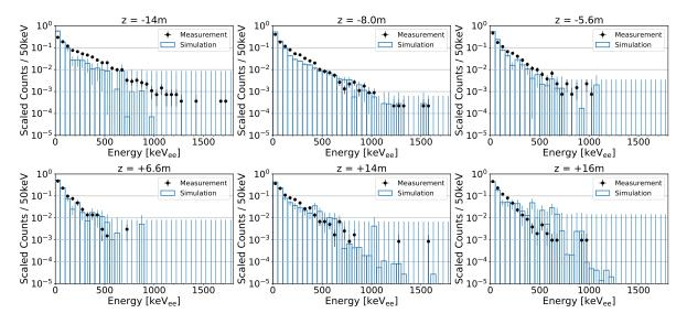
Figure 4.10: (color online) Comparison of observed (black points) and predicted (blue bars) recoil energy spectra in each TPC. The data shown are from the beam decay luminosity study periods from Study A. The lowest energy bin only includes events above the X-ray veto threshold listed in Table 4.3 in both measurement and simulation. Both distributions are normalized to an integral of unity. The title of each plot indicates the z location of its corresponding TPC.
