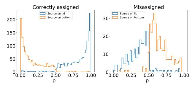
Figure 7.14: Illustration of the head-tail assignment asymmetry on simulated He recoils with reconstructed ionization energies between  $10 \text{ keV}_{ee}$  and  $20 \text{ keV}_{ee}$ . The training sample is roughly symmetric in terms of number of events with truth direction in each  $\phi_{\text{truth}}$  hemisphere, but the trained 3DCNN misassigns more events for the source-on-bottom sample than the source-on-lid sample.
