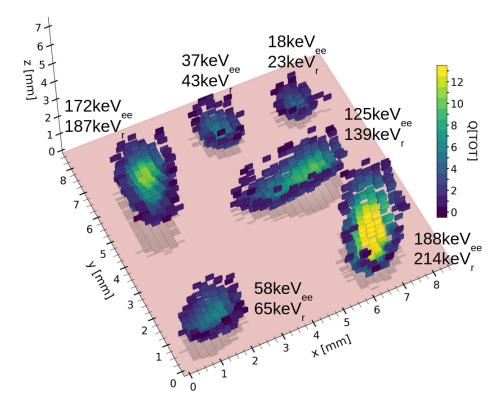
Figure 5.2: 3D charge distributions of six simulated He recoil tracks shown in the same event display. Each track is labeled with the reconstructed ionization energy (in  $keV_{ee}$ ) and true ionization energy (in  $keV_r$ ).
