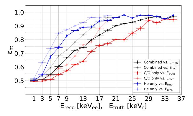
Figure 7.16: 3DCNN-determined head-tail recognition efficiencies on simulated nuclear recoils versus reconstructed nuclear recoil energy (pale colors; units in keV<sub>ee</sub>) and true ionization energy (bold colors; units in keV<sub>r</sub>). In each sample, we compute  $w = 2|p_- - 1/2|$  that corresponds to a nuclear recoil efficiency of 50% and compute  $\varepsilon_{ht}$  after these selections.
