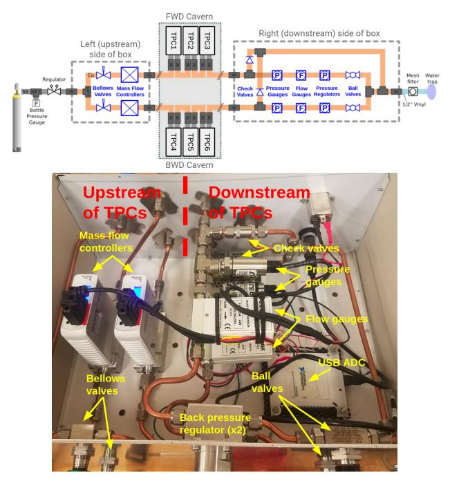
Figure 3.2: Top: Schematic of the Phase 3 gas system [not to scale]. The components shown within the bold gray dashed lines are contained within the custom-designed Gas Box. We used the same Gas Box in both Phases 2 and 3. Bottom: Inside of the Gas Box.
