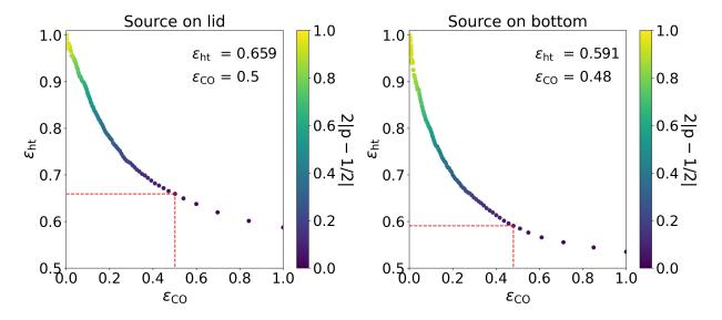
Figure 7.15: ROC curves for C/O recoil samples. Like with the He sample, despite nearly identical recoil energy spectra between the two samples (Figure 7.8), we find that performance is asymmetric and favors the source-on-lid sample.
