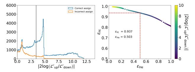
Figure 5.13: Left: Absolute value of the normalized log-likelihood ratios, with events with correctly assigned head-tail in blue and incorrectly assigned vector direction in orange. The vertical black line at  $|2\log(\mathcal{L}'_{up}/\mathcal{L}'_{down})| = 3.4$  is the 50% He recoil efficiency line. We find that nearly 94% of events with  $|2\log(\mathcal{L}'_{up}/\mathcal{L}'_{down})| > 3.4$  have correctly assigned vector direction.
