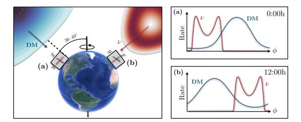
Figure 1.2: From Ref. [12]: Orientations of DM-induced and  $CE\nu NS$ -induced nuclear recoils observed in a terrestrial detector spaced 12 hours apart. The neutrino and DM-recoil signals will oscillate over the day as a function of  $\phi$  but will remain distinct from one another.
