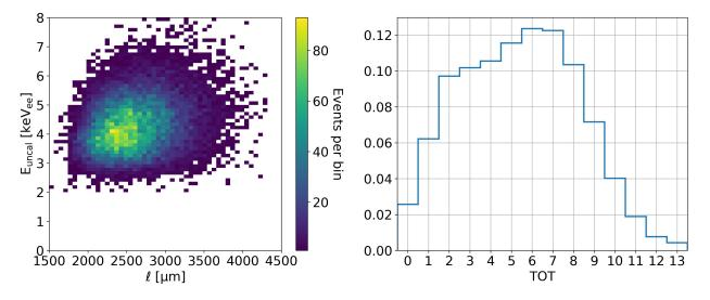
Figure 7.6: Left: Uncalibrated energy versus track length distribution of  ${}^{55}$ Fe X-rays recorded over this 8 hour period. Right: Normalized TOT distribution of all pixel hits from this sample. The low frequency of TOT = 13 hits suggests that events on average do not have significant fractions of saturated pixel hits.
