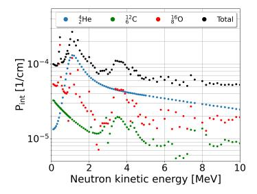
Figure 3.3: Neutron interaction probability per centimeter ( $P_{int}$ ) of gas traversed versus neutron kinetic energy in a 70:30 mixture of He:CO<sub>2</sub> at 1 atm pressure. Elastic scattering cross sections to produce this figure were obtained from the ENDF/B-VII database [67] and may differ slightly from those listed in the G4NDL4.6 library.
