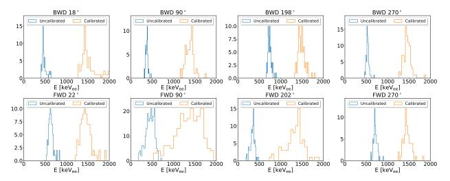
Figure 3.4: Ionization energy distributions of calibration alphas that are within  $\pm 2^{\circ}$  of both the mean  $\theta_{\rm TPC}$  and  $\phi_{\rm TPC}$  in each TPC before and after gain calibrations. We assume an uncalibrated gain of 2,000 leading to the distributions labeled "Uncalibrated" in each plot. The calibrated gains that lead to the distributions labeled "Calibrated" in each plot are listed in Table 3.1.
