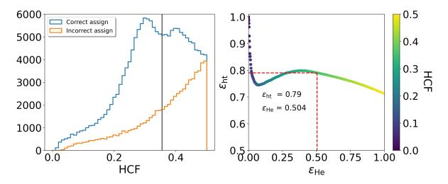
Figure 5.12: Left: HCF distributions with correctly assignments in blue and incorrect assignments in orange. The vertical black line shows the HCF value corresponding to  $\varepsilon_{\text{He}} = 0.5$ . Right: ROC curve showing  $\varepsilon_{\text{ht}}$  versus  $\varepsilon_{\text{He}}$  at various HCF selections. About 79% of events with HCF < 0.355 have correctly assigned vector direction.
