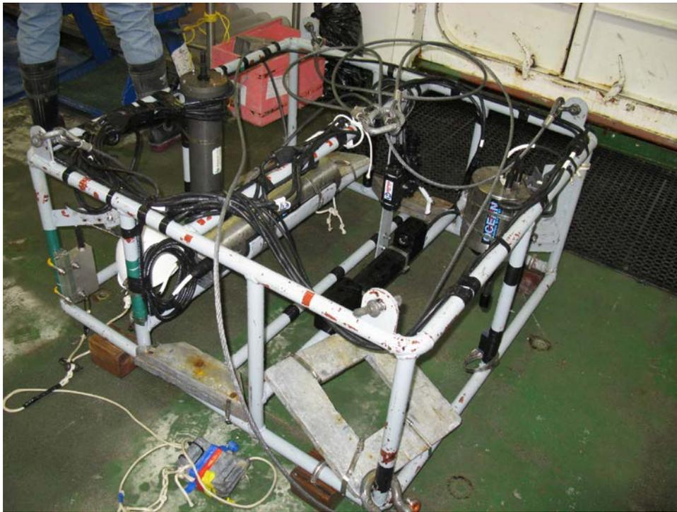
Figure 2.3: Yoyo Camera frame pre-deployment stage aboard the RV/IB-NBP. Shown in the image are the underwater camera (far right), strobe (far left), scaling lasers and bottom contact switch (center), and weighted 1.5 m lanyard (bottom center).
