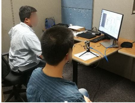
Figure 2.8 Multiple subject presence in front of the radar system. The equidistant subjects are in seated position in front of the radar at 0.5 m from radar. From [18]
