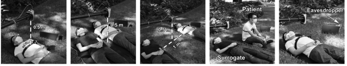
Figure 6.6 Left to right: (a) One person scenario for compliance tracking with patient; (b) Mix-up: patient lies together with non-patient in close distance; (c) Mix-up: patient lies separately with non-patient; (d) Surrogate: radar tracks non-patient; (e) Eavesdropper records signal from radar.
