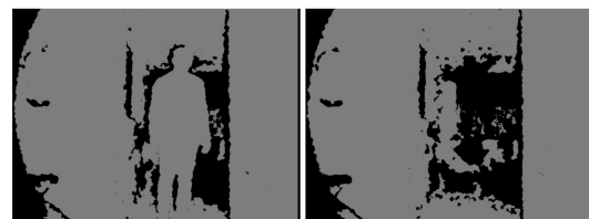
Figure 1: RGB-D Images captured by robot: Left – a person is clearly visible; Right – no person in sight.
