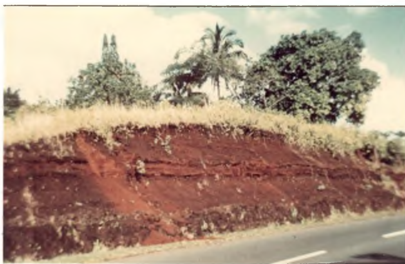
Figure 3: Banding of gibbsite in Hilo soil .
