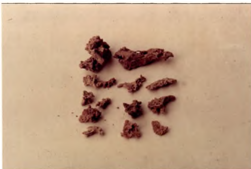
Figure 4b; Aggregated gibbsite separated from gibbsite band.
