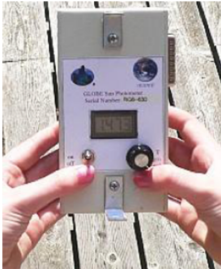
Figure 9: GLOBE sun photometer. A toggle switch on the right-hand side allows the user to switch between the red and green channels as well as the internal temperature sensor.
