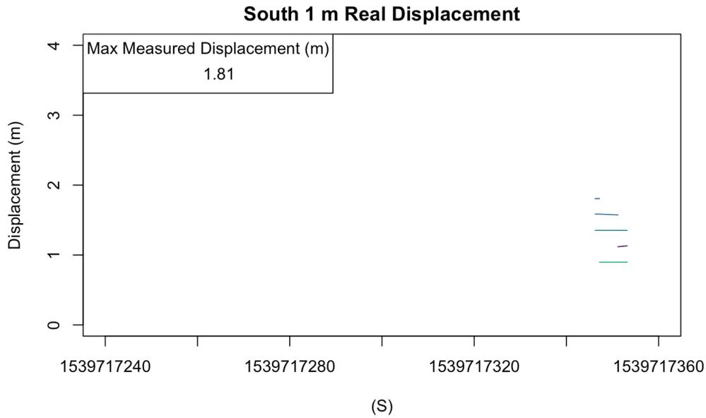
**Figure 45** Measured displacements from the UBLOX GNSS chip while the window was facing South during the 1 m real displacement. The max measured displacement after looping through lags of 1-60 seconds was 1.8 m. These results are a false positive.
