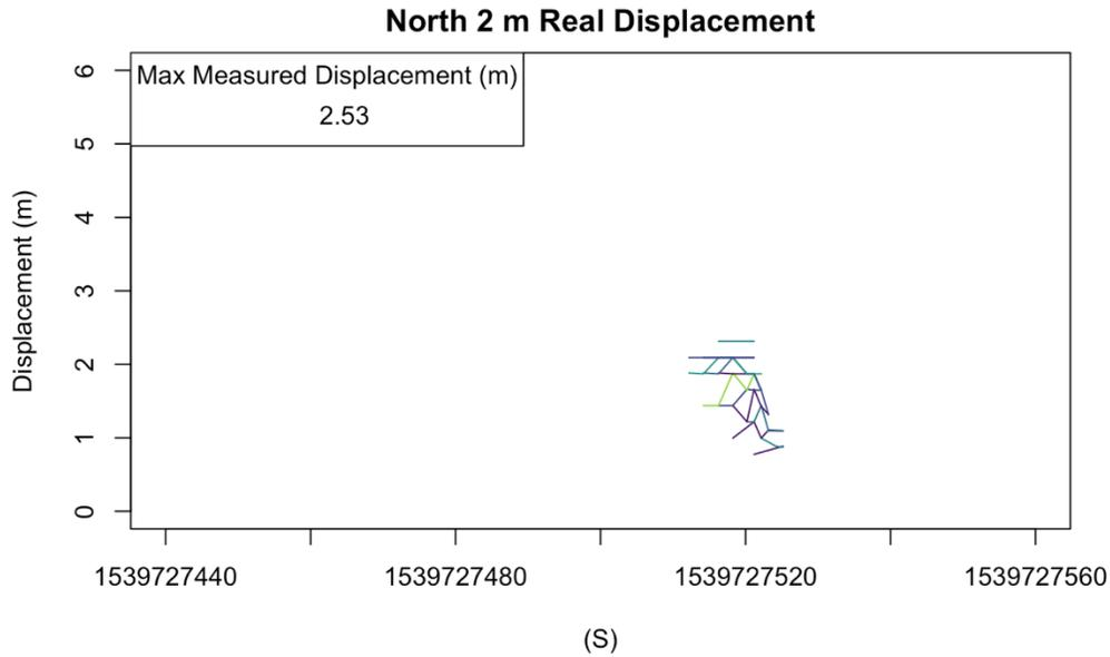
**Figure 43** Measured displacements from the UBLOX GNSS chip while the window was facing North during the 2 m real displacement. The max measured displacement after looping through lags of 1-60 seconds was 2.53 m.
