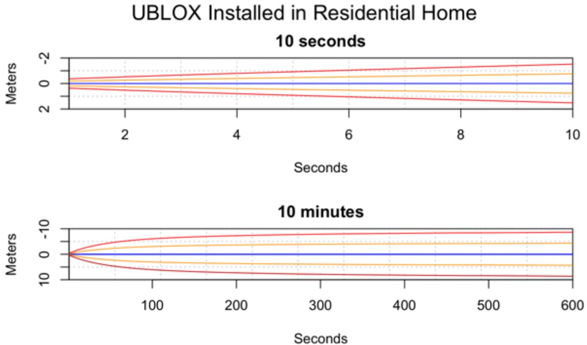
**Figure 11** Latitude difference plots over 10 seconds and 10 minutes for UBLOX GNSS chip installed in a residential home. The blue line shows the mean difference, the orange lines shows sd from the mean, and the red lines show 2sd from the mean.
