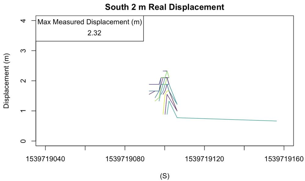
**Figure 46** Measured displacements from the UBLOX GNSS chip while the window was facing South during the 2 m real displacement. The max measured displacement after looping through lags of 1-60 seconds was 2.32 m.
