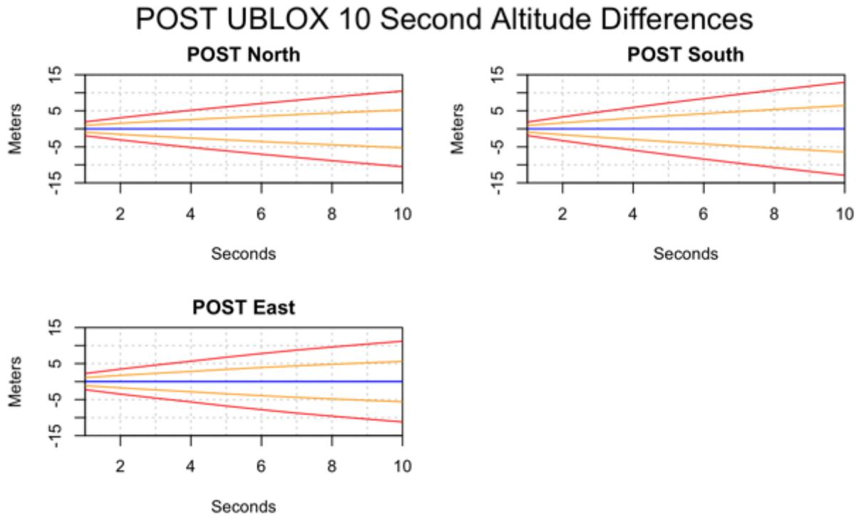
**Figure 21** Altitude difference plots over 10 seconds for the UBLOX GNSS chip installed inside the POST building. The blue line shows the mean difference, the orange lines show  $\pm 1$  standard deviation from the mean, and the red lines show  $\pm 2$  standard deviations from the mean.
