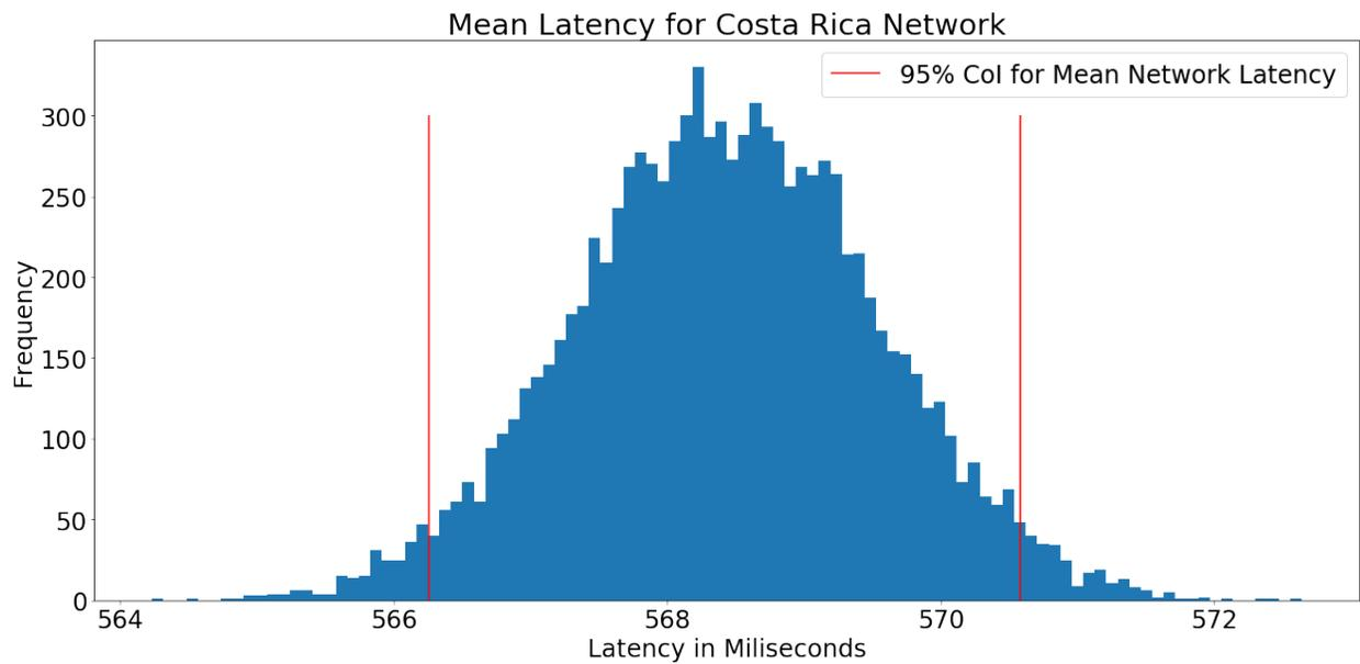
**Figure 69** 95% confidence interval for the bootstrapped mean latencies of the Costa Rica network.
