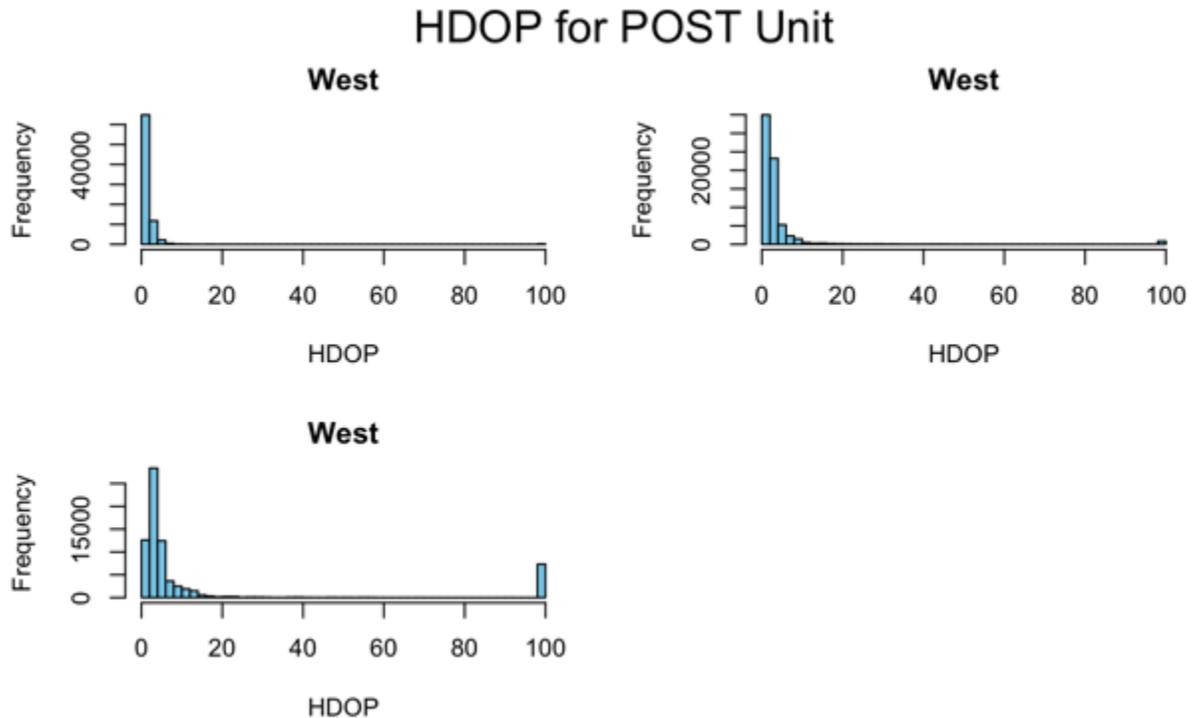
**Figure 33** Histograms of the horizontal dilution of precision for the three days the UBLOX GNSS chip that was installed inside of the POST building collected data. The reported values are within the same range for all three days.
