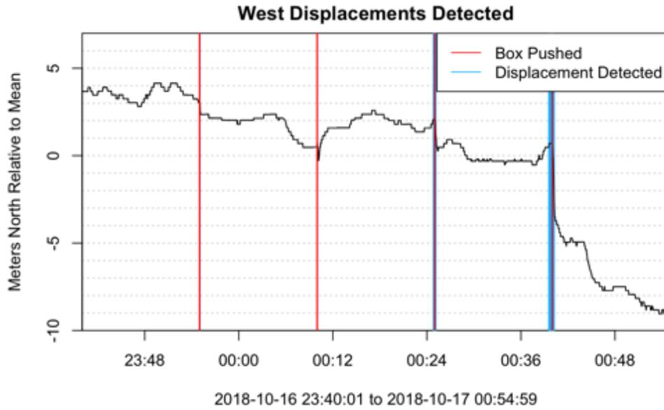
**Figure 41** Detected displacements while the window was facing West. There were no false positives, and displacements were detected during the 1 m, 2 m, and 4 m displacements.
