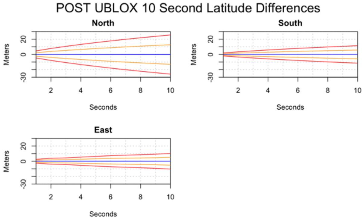
**Figure 12** Latitude difference plots over 10 seconds for the UBLOX GNSS chip installed in the POST building. The blue line shows the mean difference, the orange lines show 1sd from the mean, and the red lines show 2sd from the mean.
