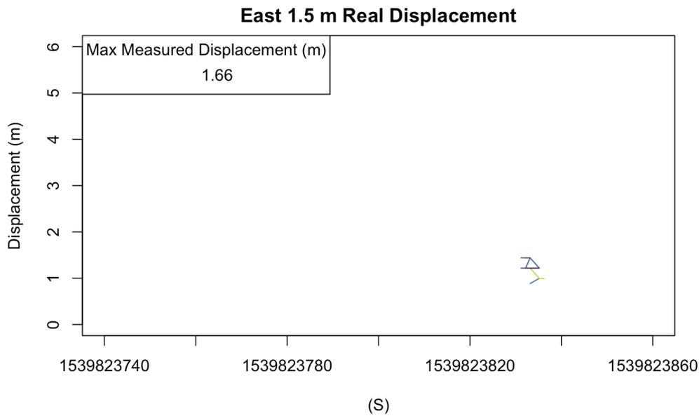
**Figure 49** Measured displacements from the UBLOX GNSS chip while the window was facing East during the 1.5 m real displacement. The max measured displacement after looping through lags of 1-60 seconds was 1.66 m.
