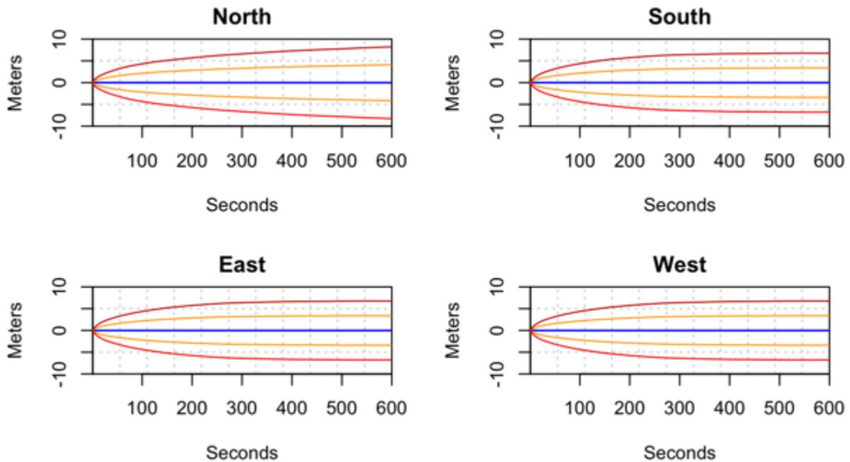
**Figure 10** Latitude difference plots over 10 minutes for the phone's internal GNSS chip installed inside the box. The blue line shows the mean difference, the orange lines show one sd from the mean, and the red lines show 2sd from the mean.
