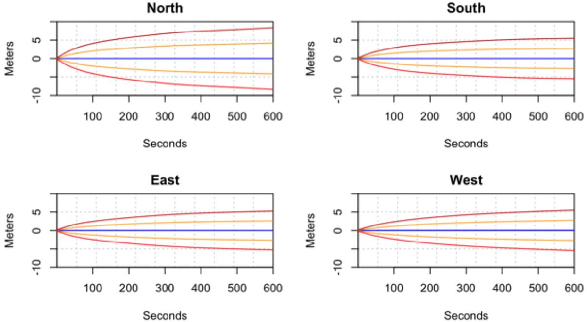
**Figure 8** Latitude difference plots over 10 minutes for the UBLOX GNSS chip installed inside the box. The blue line shows the mean difference, the orange lines show one sd from the mean, and the red lines show 2sd from the mean.
