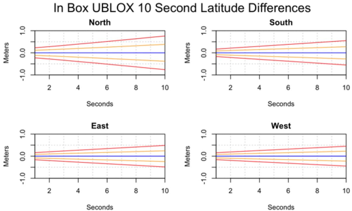
**Figure 7** Latitude difference plots over 10 seconds for the UBLOX GNSS chip installed inside the box. The blue line shows the mean difference, the orange lines shows one sd from the mean, and the red lines show 2sd from the mean.
