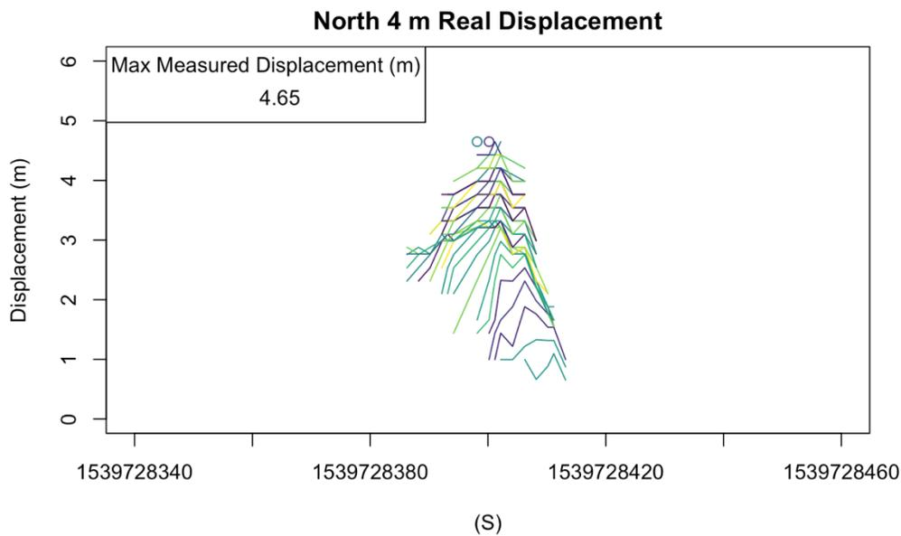
**Figure 44** Measured displacements from the UBLOX GNSS chip while the window was facing North during the 4 m real displacement. The max measured displacement after looping through lags of 1-60 seconds was 4.65 m.
