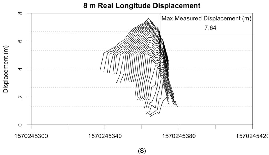
**Figure 67** Measured longitude displacements during the real 8 m displacement by the UBLOX GNSS chip. The max longitude displacement that it measured was 7.64 m.
