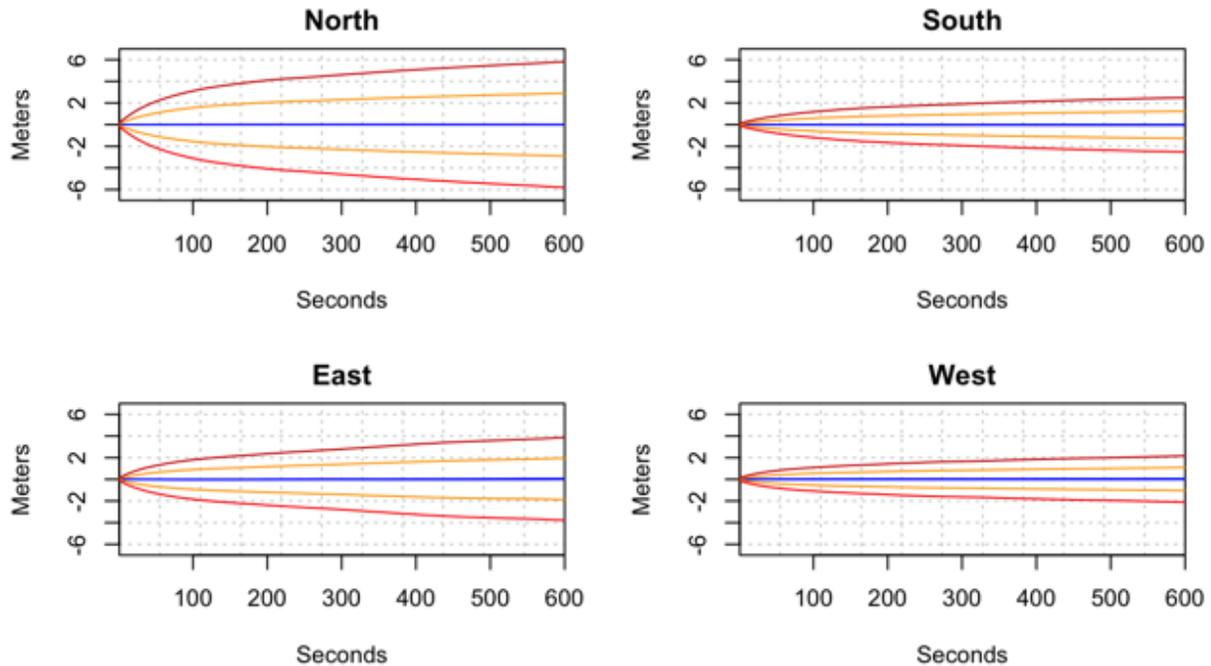
**Figure 6** Latitude difference plots over 10 minutes for the UBLOX GNSS chip installed on the roof. The blue line shows the mean difference, the orange lines show 1sd from the mean, and the red lines show 2sd from the mean.
