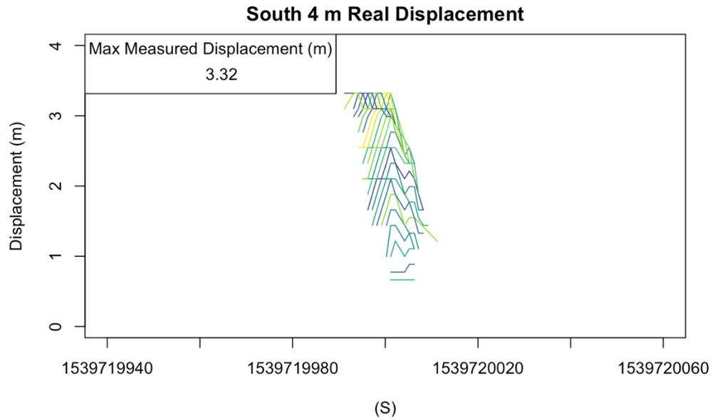
**Figure 47** Measured displacements from the UBLOX GNSS chip while the window was facing South during the 4 m real displacement. The max measured displacement after looping through lags of 1-60 seconds was 3.32 m.
