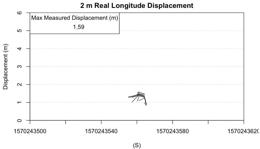
**Figure 65** Measured longitude displacements during the real 2 m displacement by the UBLOX GNSS chip. The max longitude displacement that it measured was 1.59 m.
