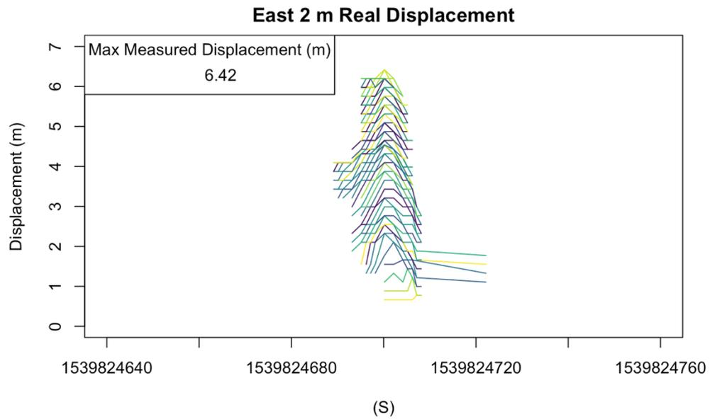
**Figure 50** Measured displacements from the UBLOX GNSS chip while the window was facing East during the 2 m real displacement. The max measured displacement after looping through lags of 1-60 seconds was 6.42 m. This was the largest outlier seen during the test.
