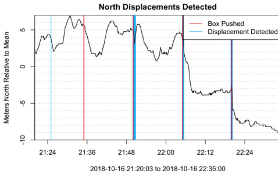
**Figure 38** Detected displacements while the window was facing North. There was only one false positive displacement at the beginning of the test. The displacement model didn't pick up a 1 m push at the beginning of the test.
