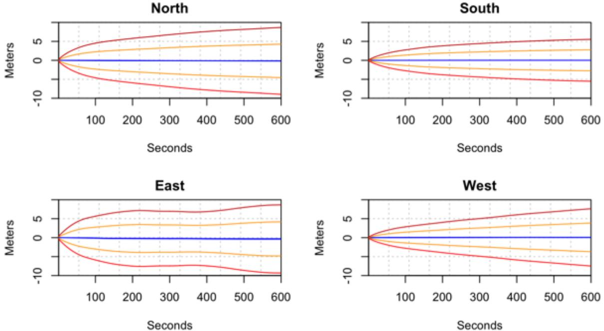
**Figure 15** Altitude difference plots over 10 seconds for the Control UBLOX GNSS chip. The blue line shows the mean difference, the orange lines show 1sd from the mean, and the red lines show 2sd from the mean.
