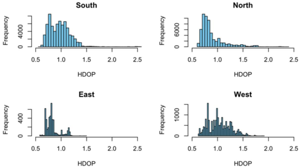
**Figure 31** Histograms of the horizontal dilution of precision for the four days the UBLOX GNSS chip which was installed on the roof collected data. There isn't a large range in the values, and the day the window was facing North showed some of the lower HDOP values.
