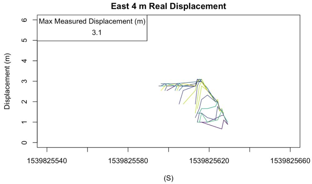
**Figure 51** Measured displacements from the UBLOX GNSS chip while the window was facing East during the 4 m real displacement. The max measured displacement after looping through lags of 1-60 seconds was 3.02 m.
