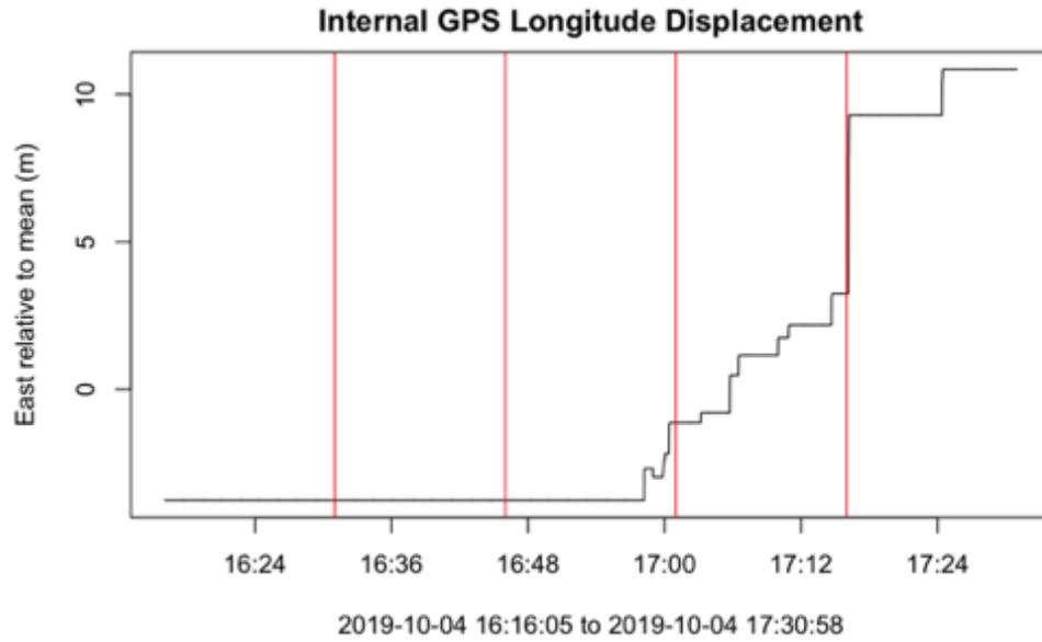
**Figure 57** Longitude displacement time series for the phones internal GNSS chip. The red lines denote the times when the box was actually pushed. The internal GNSS chip is filtering the data to keep the reported position as consistent as possible. During the longitude displacement test the box was pushed 1 m, 2 m, 4 m, and 8 m. Only the 8 m displacement was detected during the longitude displacement test.
