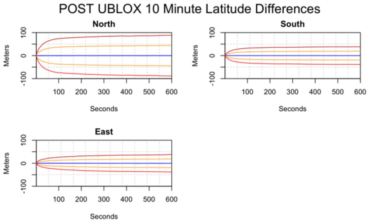
**Figure 13** Latitude difference plots over 10 minutes for the UBLOX GNSS chip installed in the POST building. The blue line shows the mean difference, the orange lines shows on sd from the mean, and the red lines show 2sd from the mean.
