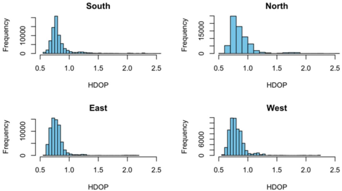
**Figure 32** Histograms of the horizontal dilution of precision for four days the UBLOX GNSS chip that was installed inside of the box collected data. The histogram for the day the window was facing North doesn't seem to be any different from the rest of the histograms.
