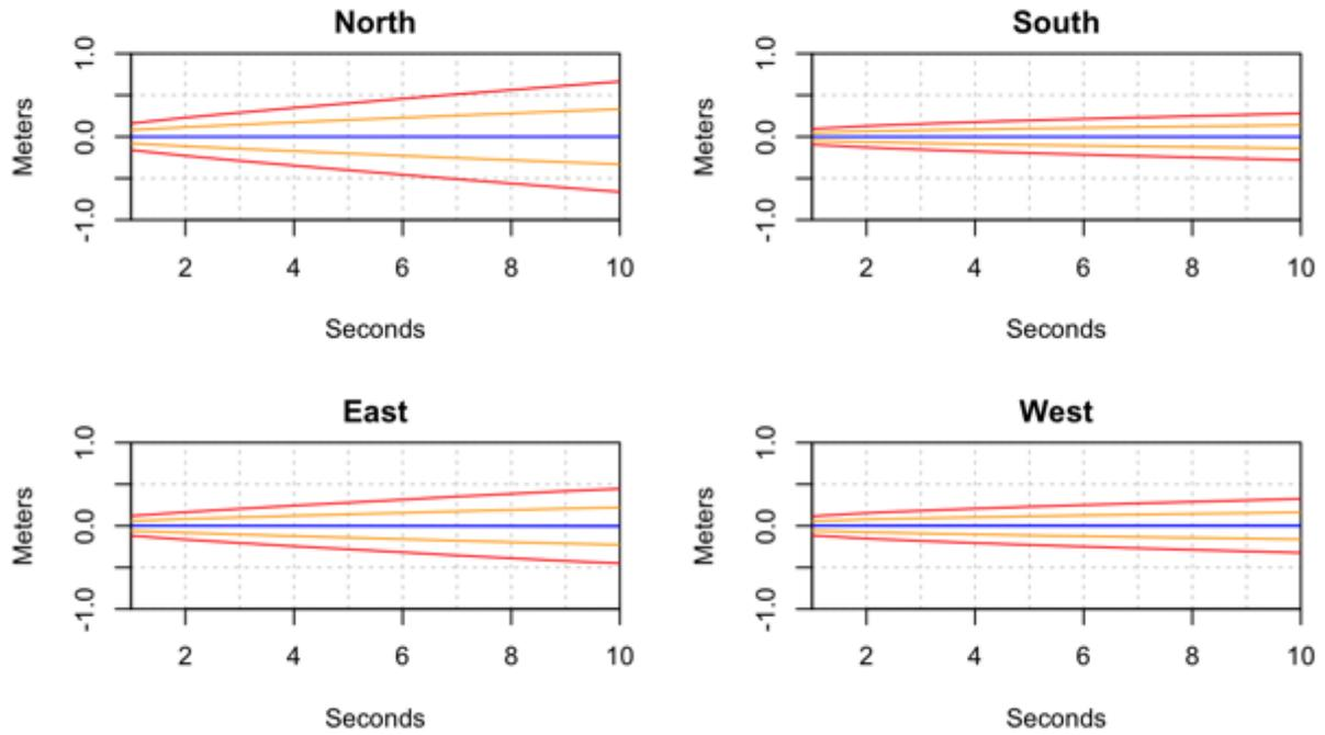
**Figure 6** Latitude difference plots over 10 seconds for the UBLOX GNSS chip installed on the roof. The blue line shows the mean difference, the orange lines show 1sd from the mean, and the red lines show 2sd from the mean.
