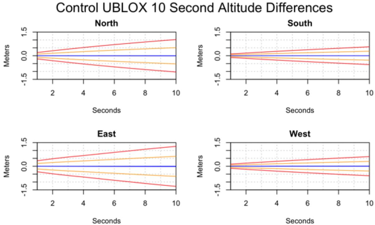
**Figure 14** Altitude difference plots over 10 seconds for the Control UBLOX GNSS chip. The blue line shows the mean difference, the orange lines show  $\pm 1\text{sd}$  from the mean, and the red lines show  $\pm 2\text{sd}$  from the mean.
