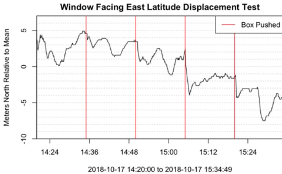
**Figure 37** Latitude displacement time series pushed with the window facing East recorded by the external UBLOX GNSS chip.
