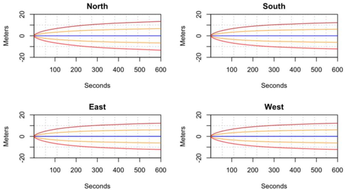
**Figure 19** Altitude difference plots over 10 minutes for the phones Internal GNSS chip installed inside the box. The blue line shows the mean difference, the orange lines shows on sd from the mean, and the red lines show 2sd from the mean.
