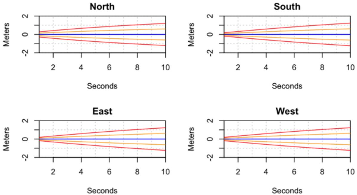
**Figure 9** Latitude difference plots over 10 seconds for the phone's internal GNSS chip installed inside the box. The blue line shows the mean difference, the orange lines shows one sd from the mean, and the red lines show 2sd from the mean.
