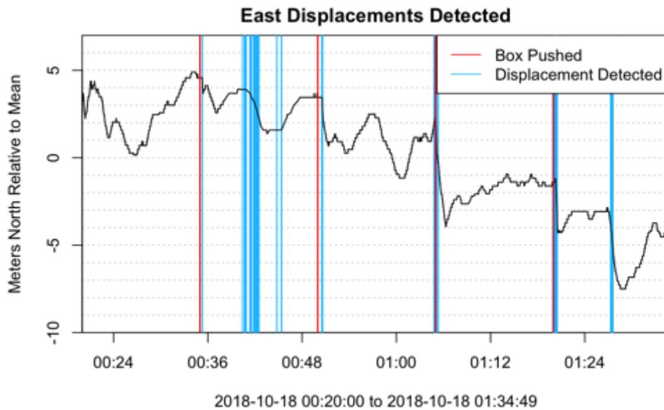
**Figure 40** Detected displacements while the window was facing East. There were several false positives, but all four displacements were detected.
