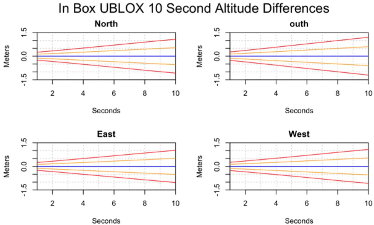
**Figure 16** Altitude difference plots over 10 seconds for the UBLOX GNSS chip installed inside the box. The blue line shows the mean difference, the orange lines shows on sd from the mean, and the red lines show 2sd from the mean.
