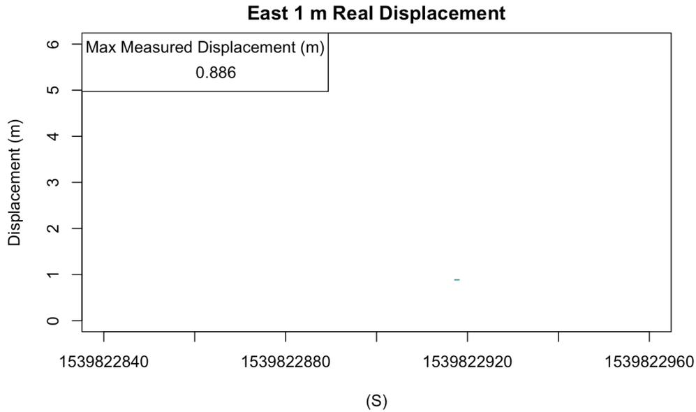
**Figure 48** Measured displacements from the UBLOX GNSS chip while the window was facing East during the 1 m real displacement. The max measured displacement after looping through lags of 1-60 seconds was 0.89 m.
