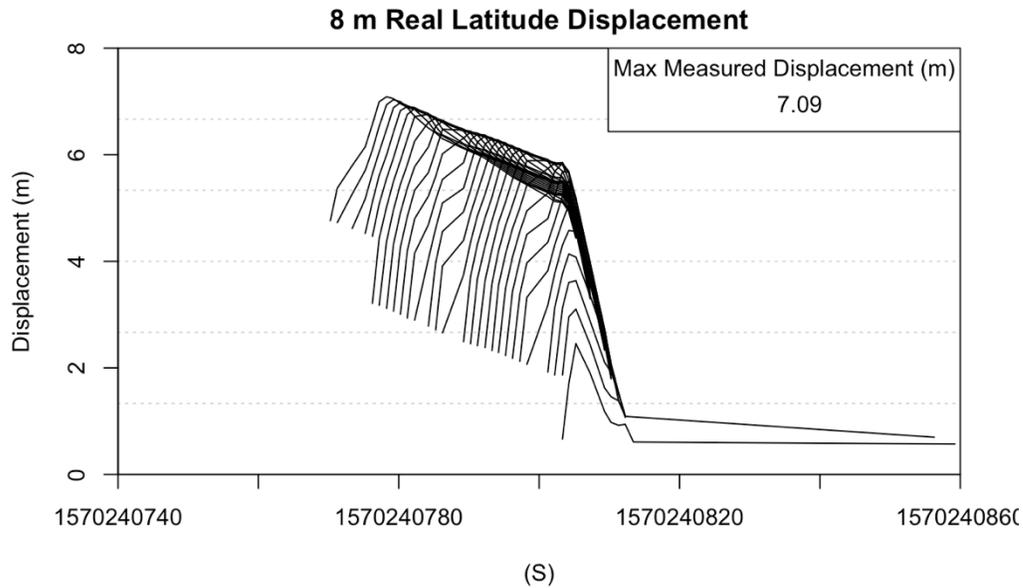
**Figure 62** The measured latitude displacement measured by the UBLOX GNSS chip during the real 8 m displacement. The max measured displacement was 7.09 m.
