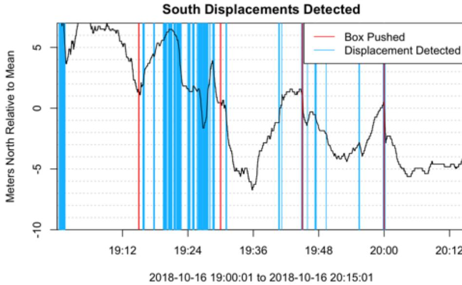
**Figure 39** Detected displacements while the window was facing South. There were much more false positives during this test. The 1 m, 2 m, and 4 m, displacements were detected by the model however.
