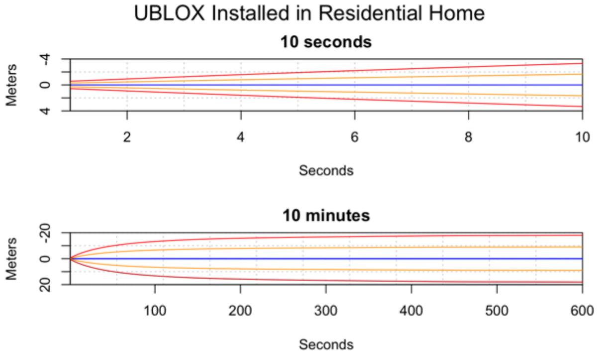
**Figure 20** Altitude difference plots over 10 seconds and 10 minutes for the GNSS UBLOX GNSS sensor that was installed in a south facing window of a residential home in Novato California. The blue line shows the mean difference, the orange lines shows on sd from the mean, and the red lines show 2sd from the mean.
