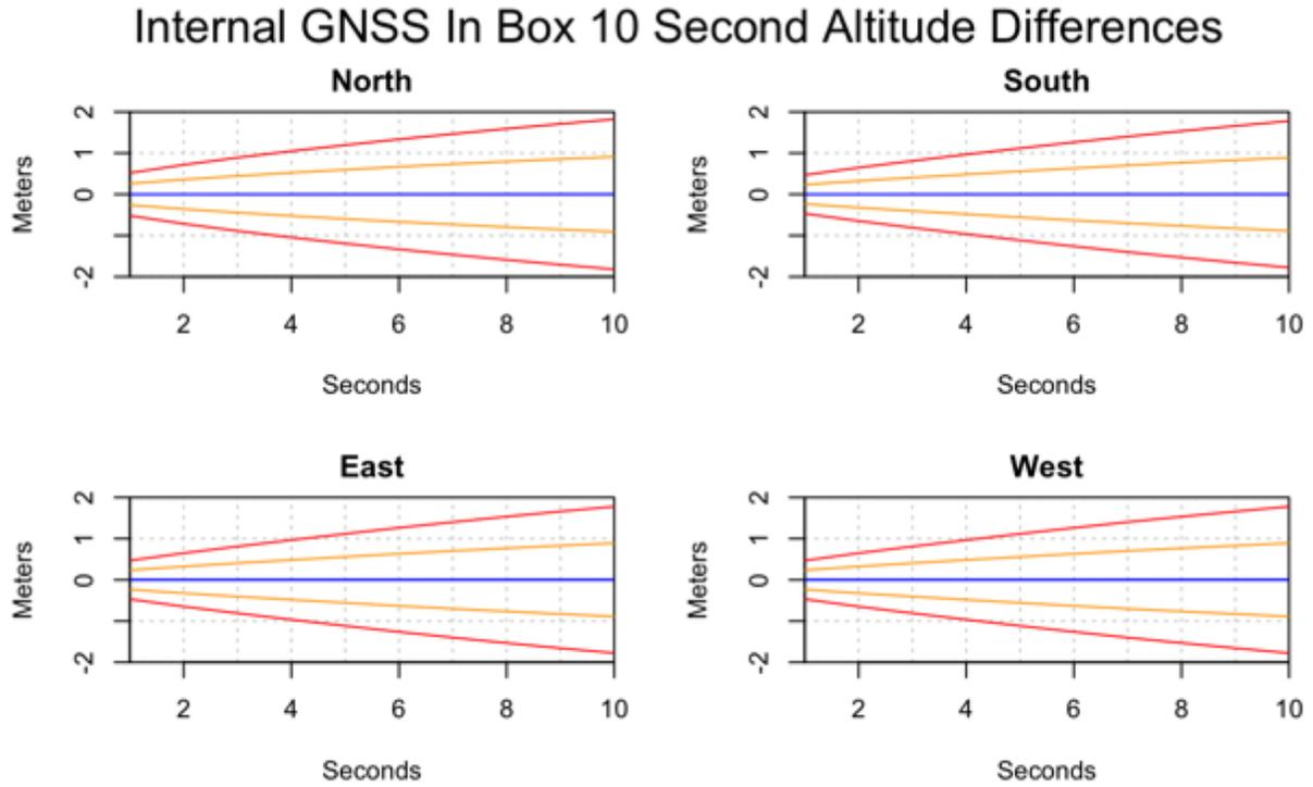
**Figure 18** Altitude difference plots over 10 seconds for the phones Internal GNSS chip installed inside the box. The blue line shows the mean difference, the orange lines shows on sd from the mean, and the red lines show 2sd from the mean.
