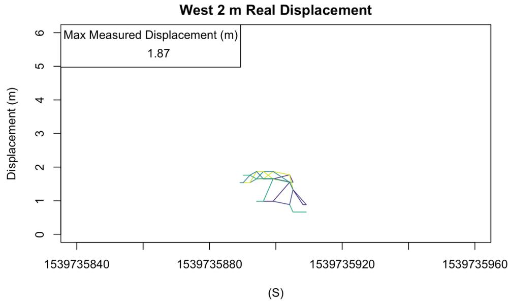
**Figure 53** Measured displacements from the UBLOX GNSS chip while the window was facing West during the 2 m real displacement. The max measured displacement after looping through lags of 1-60 seconds was 1.87 m.
