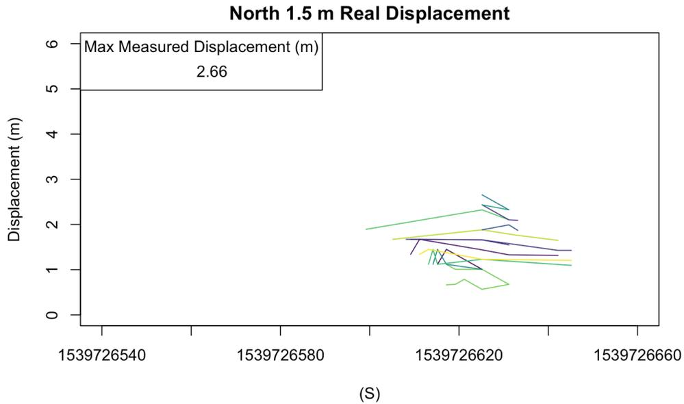
**Figure 42** Measured displacements from the UBLOX GNSS chip while the window was facing North during the 1.5 m real displacement. The max measured displacement after looping through lags of 1-60 seconds was 2.66 m.
