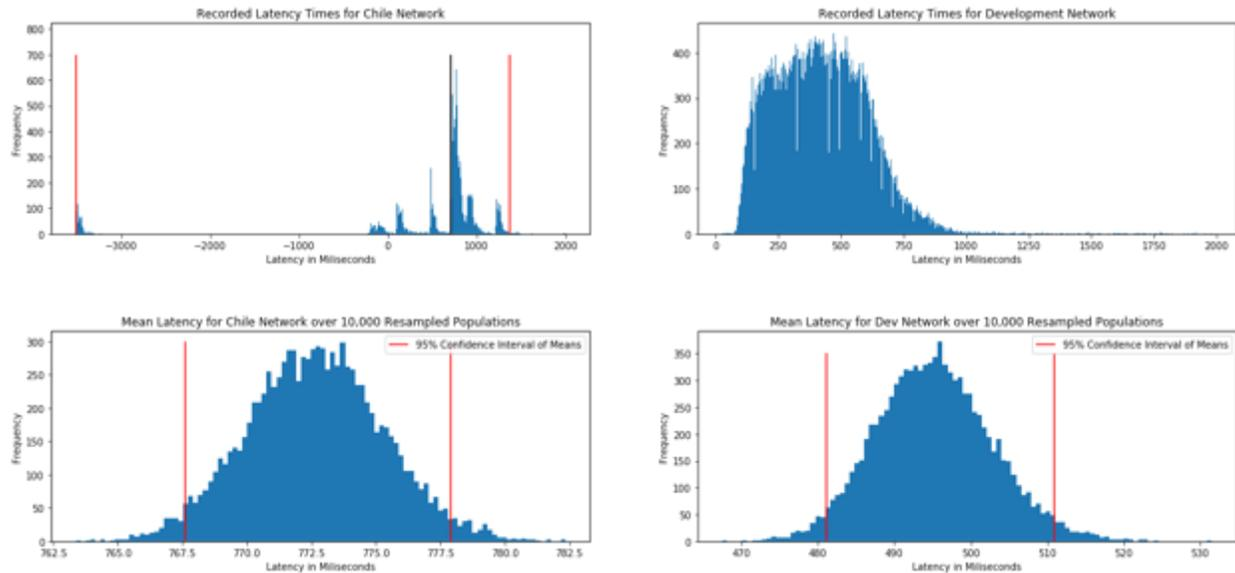
**Figure 70** Recorded latencies for the Chile network (top left) and development network (top right). The 95% confidence interval of the Chile network (bottom left) and development network (bottom right).
