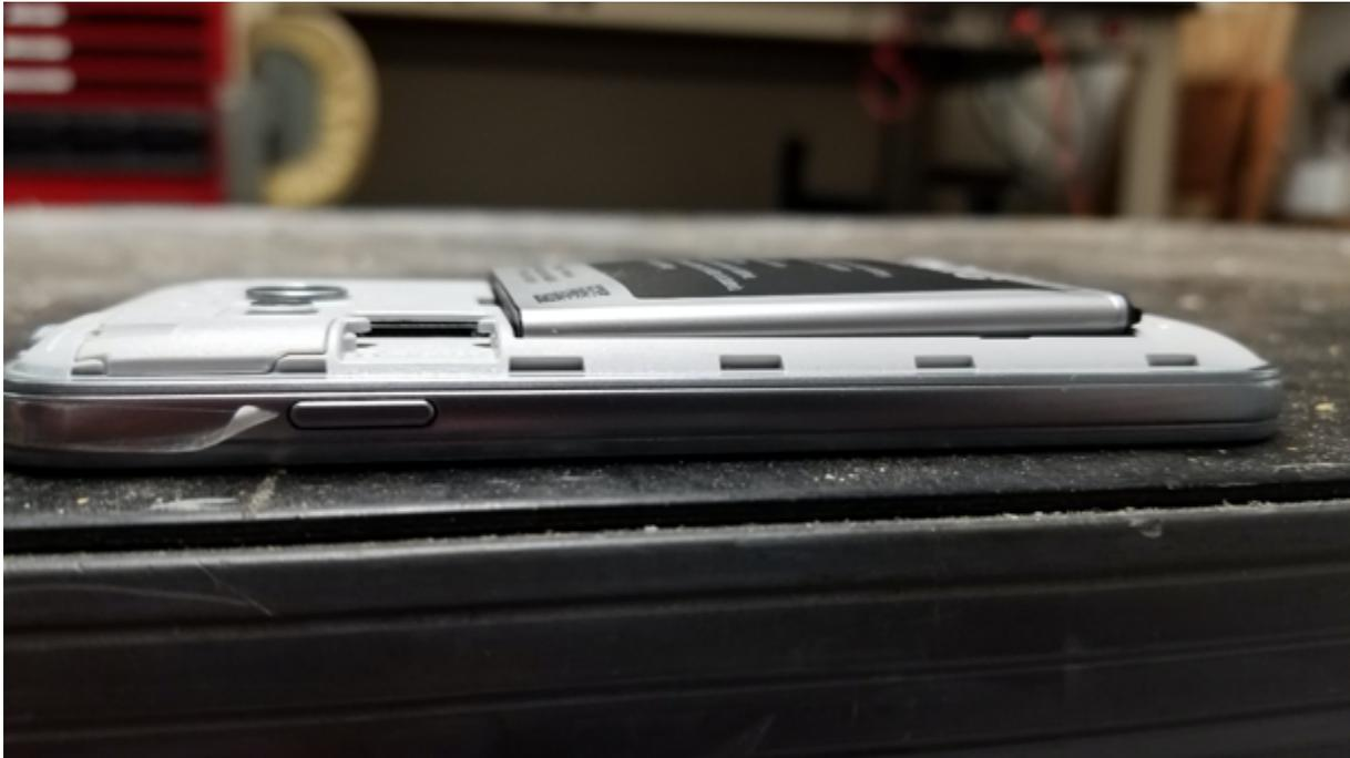
**Image 2** A swollen battery in a Samsung Ace4 Neo phone. The battery is so swollen that it will not fit in its slot, and the battery pins can't reach the corresponding pins on the phone. When this happens the back of the phone can come off and the battery will disconnect itself, or if the back can't come off then the battery will swell into the phone and crush the phones circuit board.
