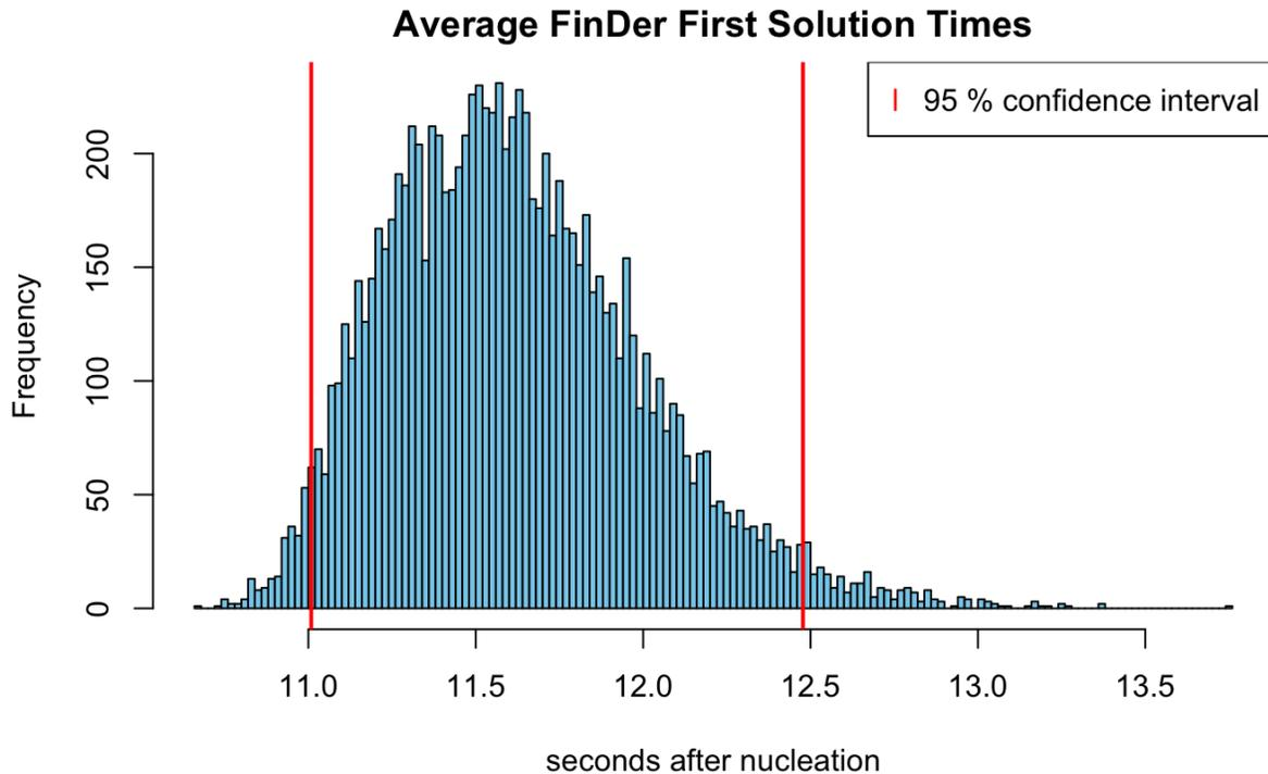
**Figure 73** The histogram of the mean solution times from FinDer over 10,000 bootstrapped samples. The 95% confidence interval for the first solution we would expect to see from the 2012 Nicoya earthquake is between 11 s, and 12.48 s. This would give warning times of 14.25-15.73 s, 18.45-19.93 s, 38.33-39.81 s for Puntarenas, Liberia, and San Jose respectively.
