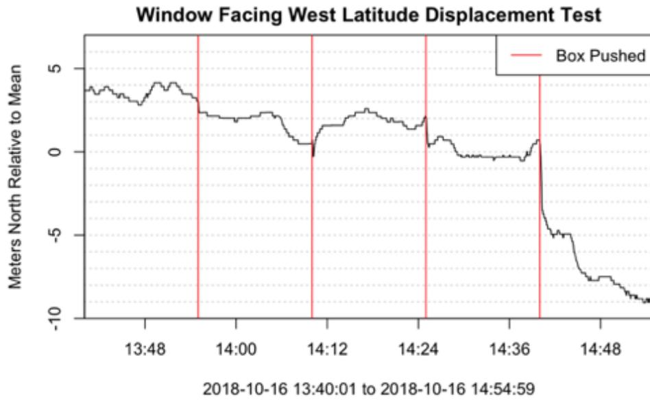
**Figure 36** Latitude displacement time series pushed with the window facing West recorded by the external UBLOX GNSS chip.
