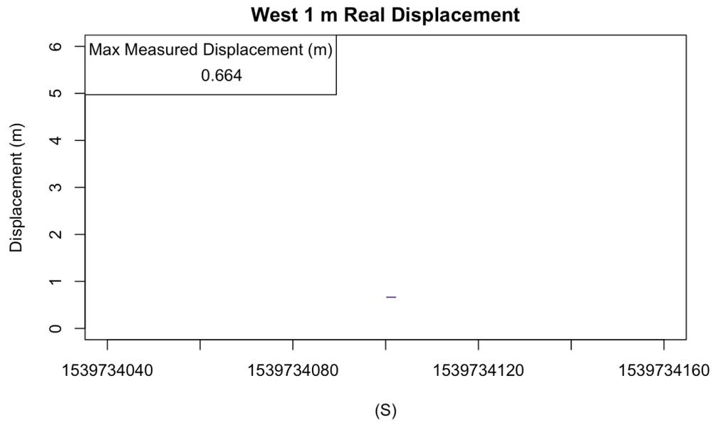
**Figure 52** Measured displacements from the UBLOX GNSS chip while the window was facing West during the 1 m real displacement. The max measured displacement after looping through lags of 1-60 seconds was 0.66 m.
