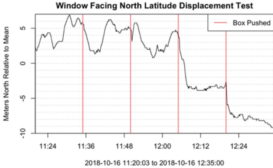
**Figure 34** Latitude displacement time series pushed with the window facing North recorded by the external UBLOX GNSS chip.
