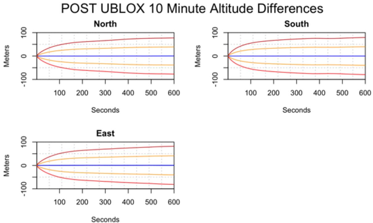
**Figure 22** Altitude difference plots over 10 minutes for the UBLOX GNSS chip installed inside the POST building. The blue line shows the mean difference, the orange lines shows on sd from the mean, and the red lines show 2sd from the mean.
