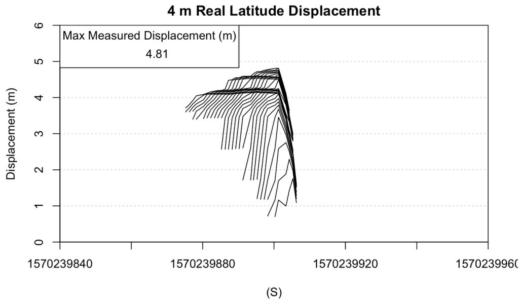
**Figure 61** The measured latitude displacement measured by the UBLOX GNSS chip during the real 4 m displacement. The max measured displacement was 4.81 m.
