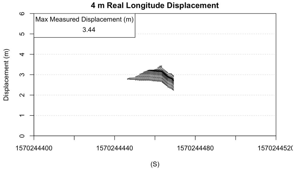
**Figure 66** Measured longitude displacements during the real 4 m displacement by the UBLOX GNSS chip. The max longitude displacement that it measured was 3.44 m.
