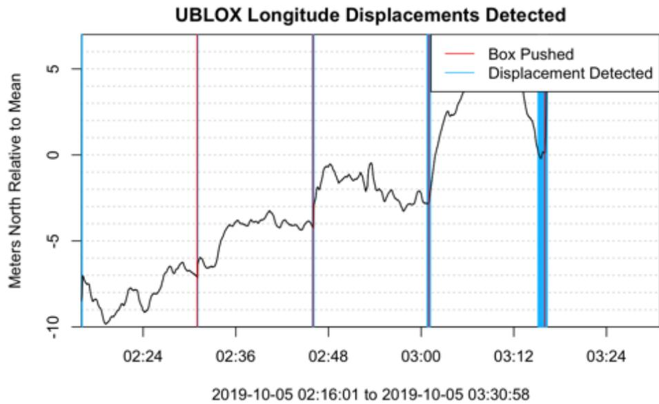
**Figure 63** The UBLOX GNSS chip longitude displacement time series. The displacement detection model was run over this second latitude displacement run, and all 4 displacements of 1 m, 2 m, 4 m, and 8 m, were detected with only a couple of false positives at the beginning of the test.
