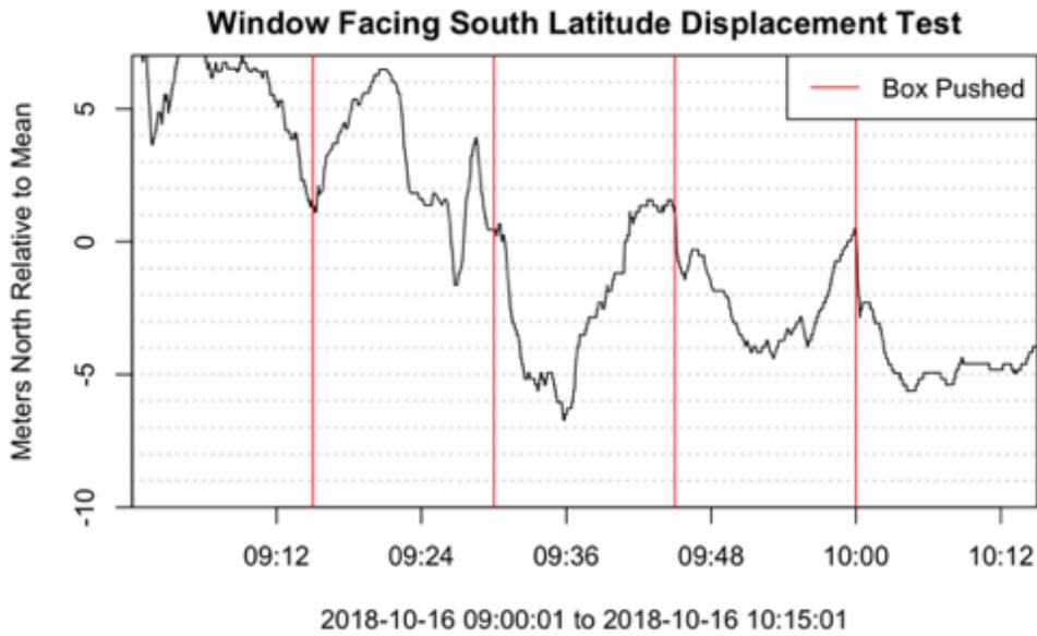
**Figure 35** Latitude displacement time series pushed with the window facing South recorded by the external UBLOX GNSS chip.
