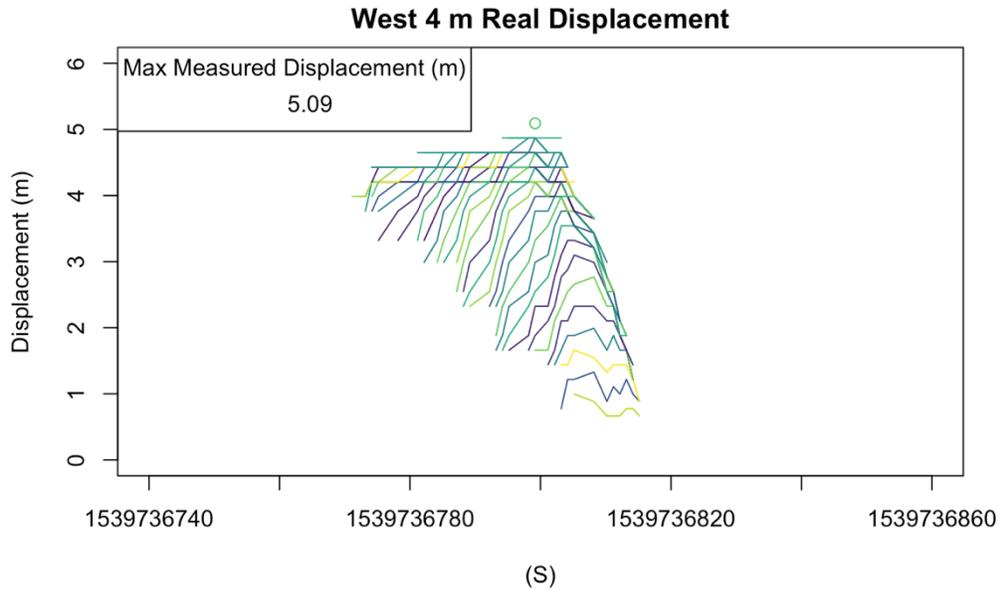
**Figure 54** Measured displacements from the UBLOX GNSS chip while the window was facing West during the 4 m real displacement. The max measured displacement after looping through lags of 1-60 seconds was 5.09 m.
