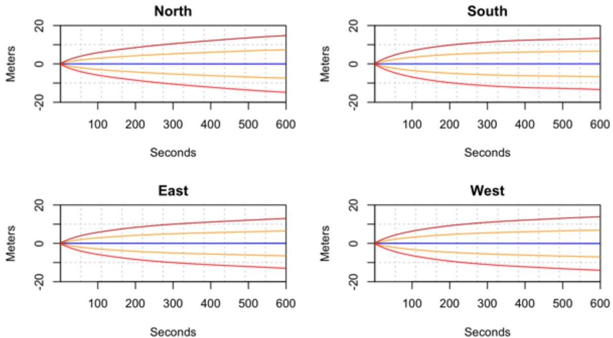
**Figure 17** Altitude difference plots over 10 minutes for the UBLOX GNSS chip installed inside the box. The blue line shows the mean difference, the orange lines show the standard deviation from the mean, and the red lines show two standard deviations from the mean.
