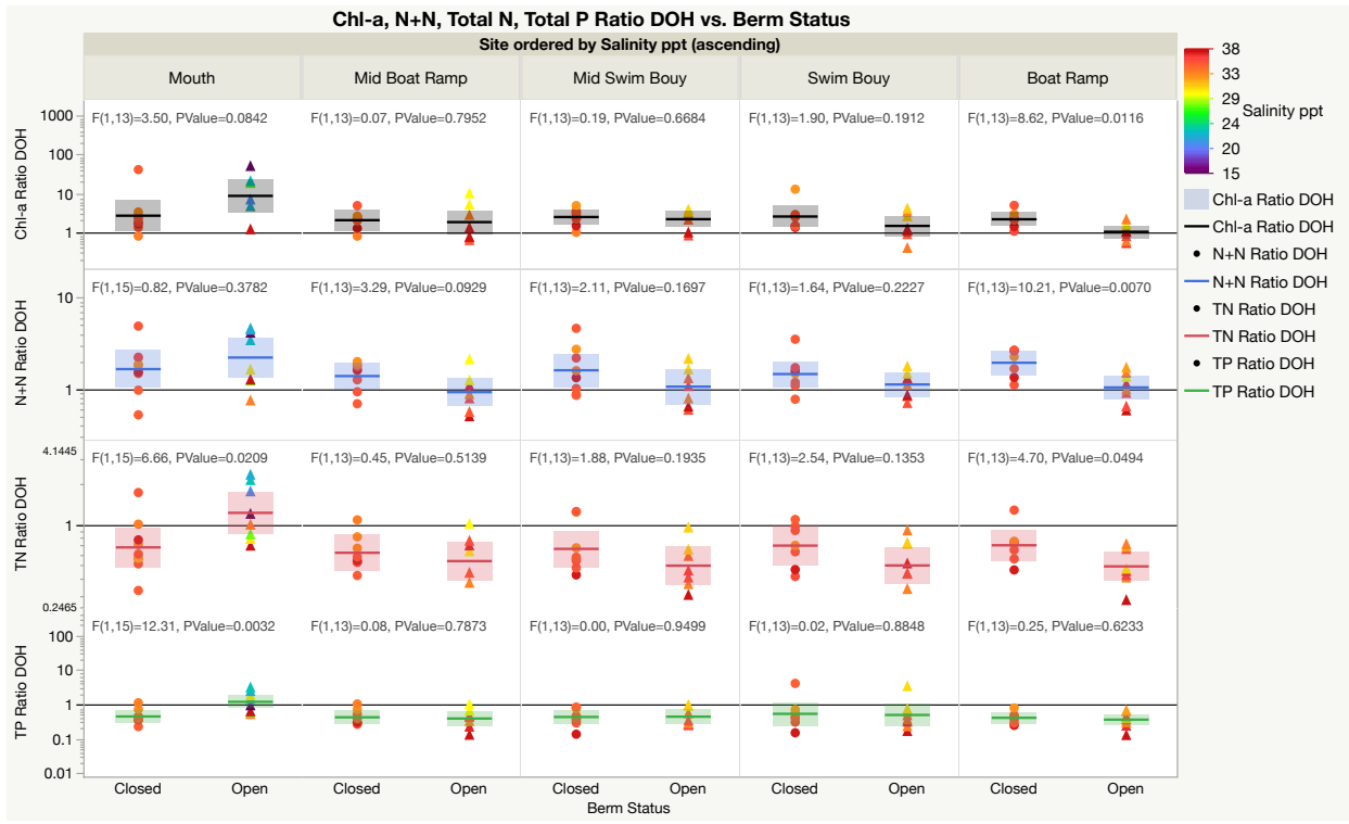
Figure 15: T-Test berm open vs. closed assessing Chlorophyll-a and Nutrients when ratio standardizing "Wet" and "Dry" conditions along the coastal waters and immediately seaward of the stream mouth is applied. There appear to be increase of Total Phosphate and Total Nitrogen explained by the presence or absence of the berm directly seaward of the stream mouth, those differences do not appear elsewhere. Values that are above 1, indicated by the line aligning with the y axis, are considered impaired by Department of Health guidelines.
