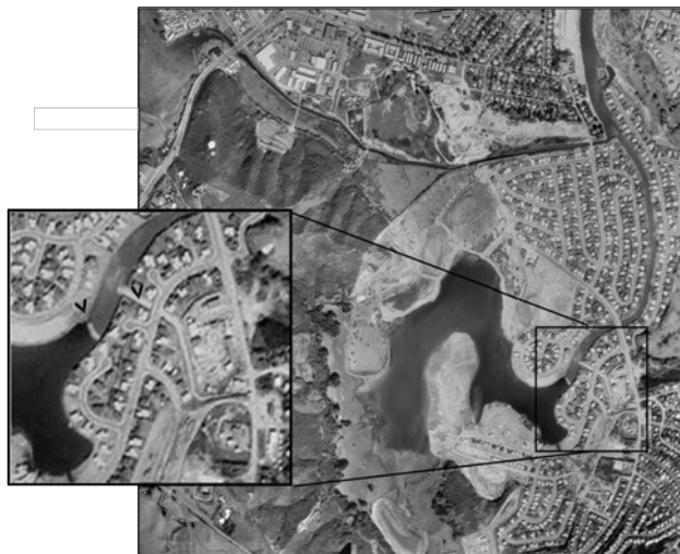
Figure 3: The dredging of Kaelepulu Pond, creation of fast land for houses and the construction of a submerged sill, restricting flow between the pond and the estuary. Credit Bourke, 2016
