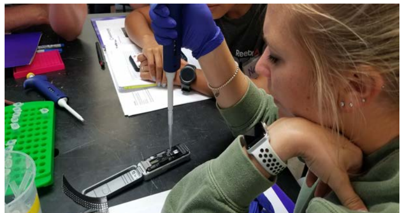
Figure 29: Teacher from Kailua Inter loads a flow cell for DNA sequencing
