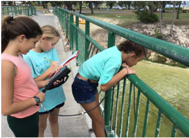
Figure 21: Students using YSI ProDSS to vertically sample Ka'elepulu Stream at Lanikai Bridge
