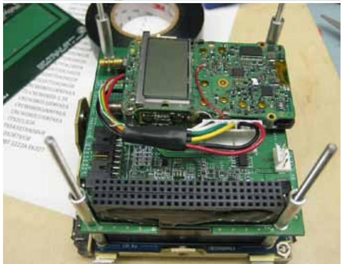
Top: CubeSat internal stack. Above: CubeSat radio and sensor board.
