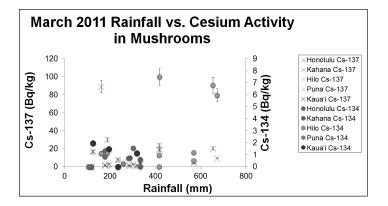
**Figure 2** March 2011 rainfall in mm vs. radiocesium activity in Bq/kg for samples collected on the islands of O'ahu and Hawai'i (both <sup>137</sup>Cs and <sup>134</sup>Cs). Activities have been decay corrected to March 2011, the month of the Fukushima disaster.
