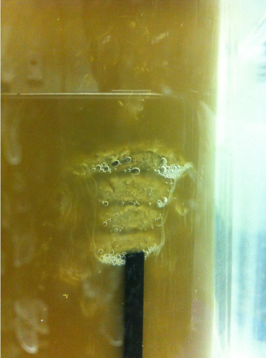
Fungal plugging between draft tube and sidewall.
