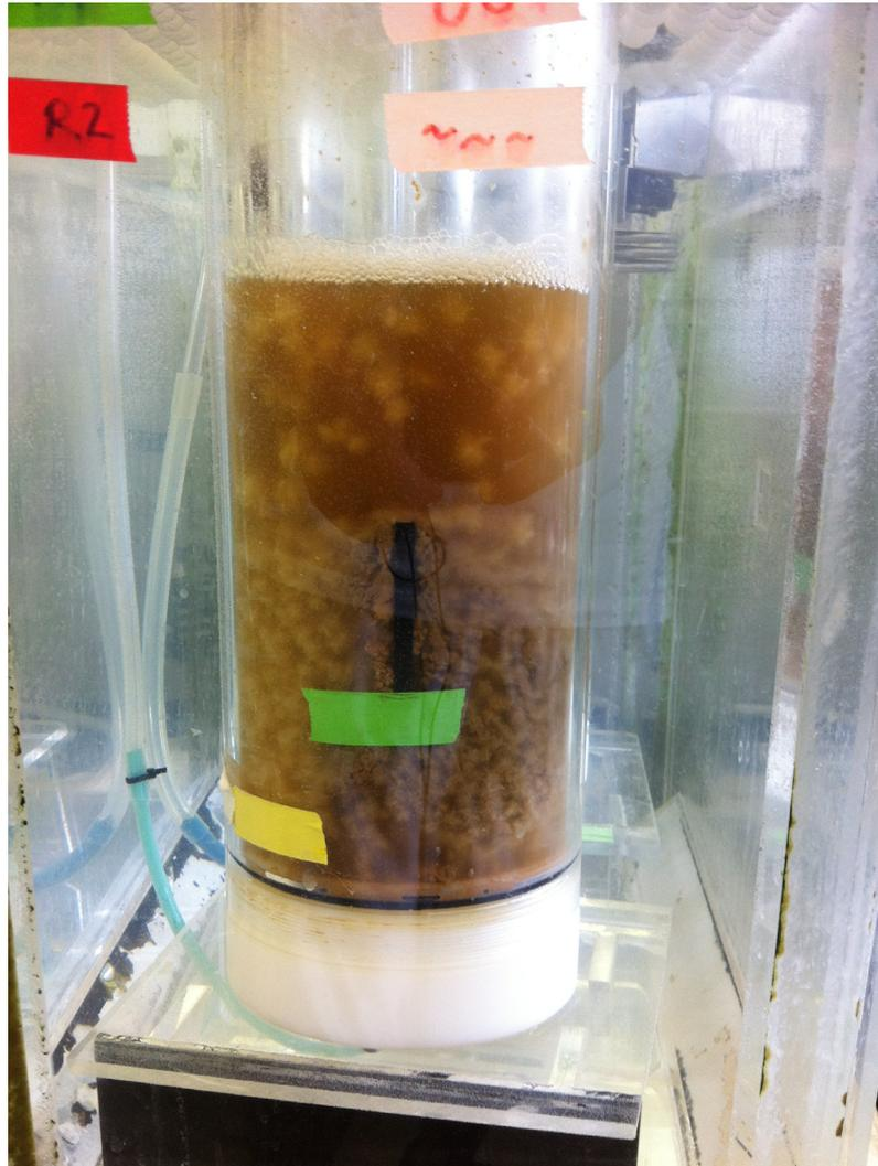
**Figure 4.1 Plugged airlift bioreactor**
