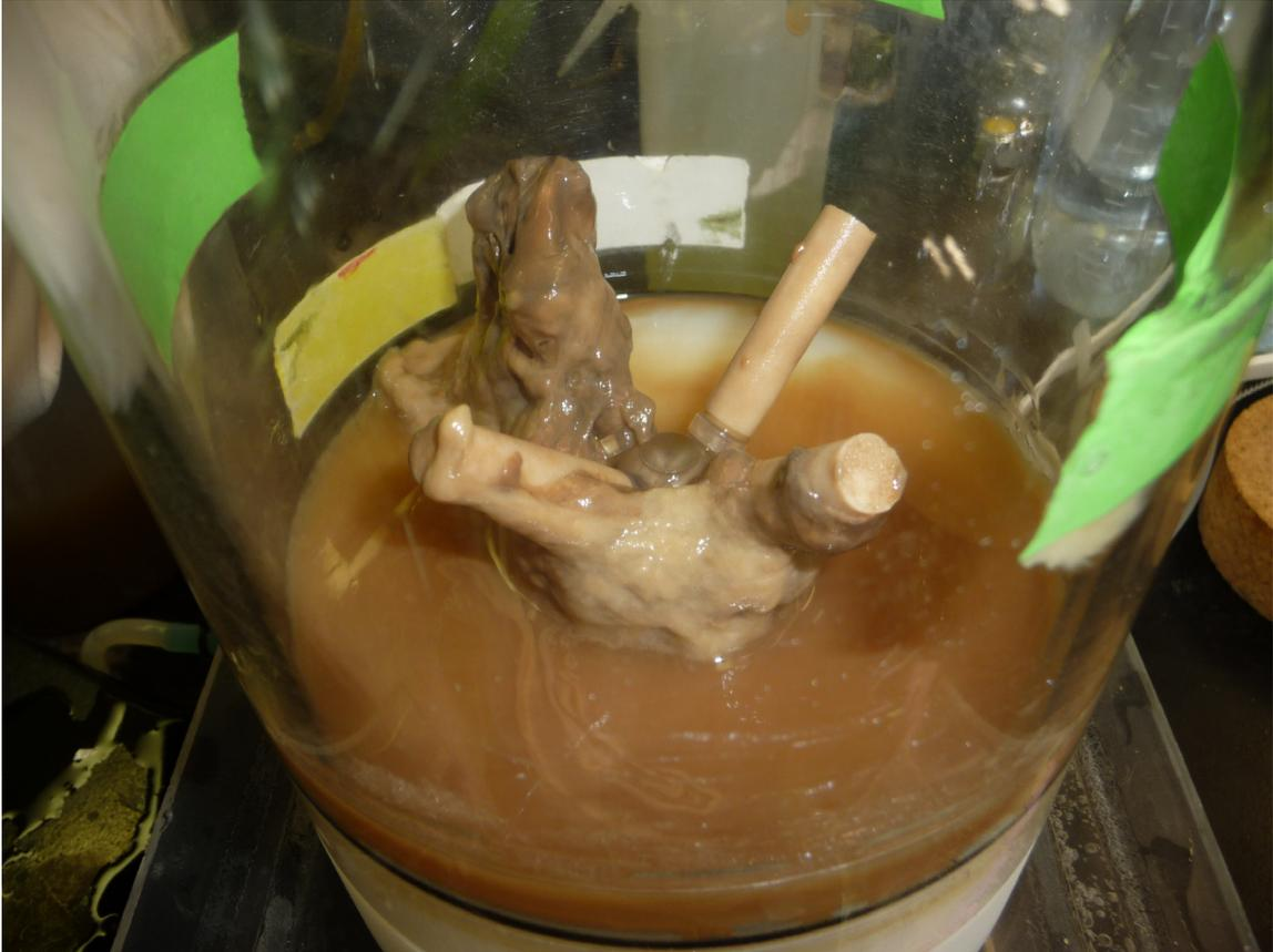
**Figure 4.10 Air diffuser fouling in airlift reactor**
