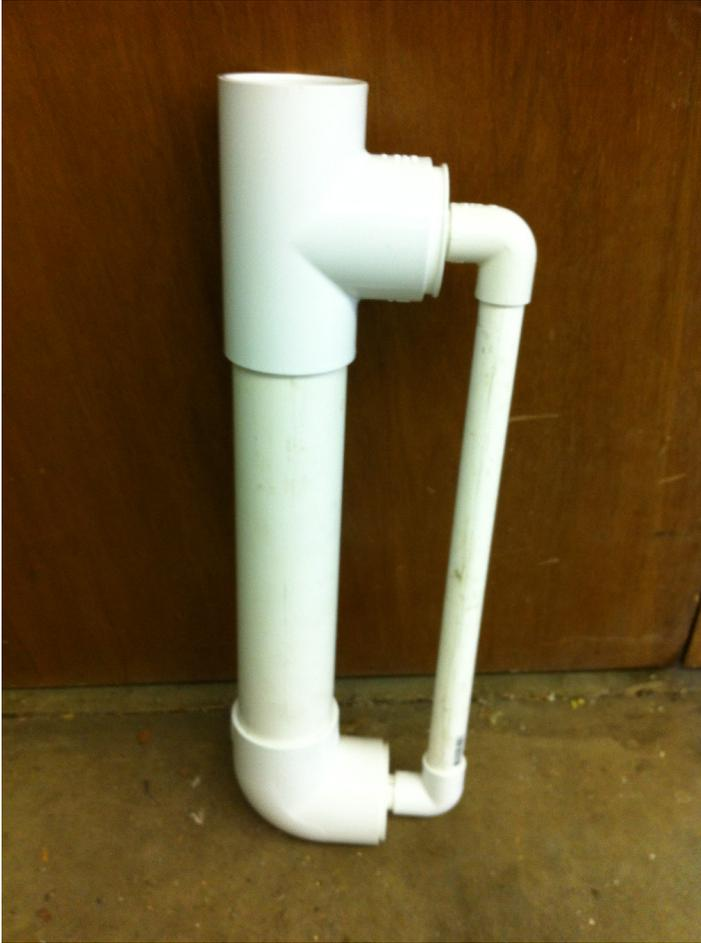
Prototype external loop airlift bioreactor, PVC pipe. Could not be heated, leaked, fungus probably would get stuck in the 1" downcomer tube.
