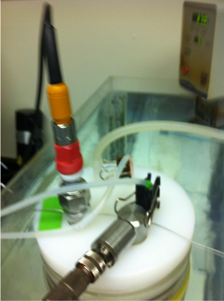
Top of airlift bioreactor. pH probe (orange) and DO probe, lower right
