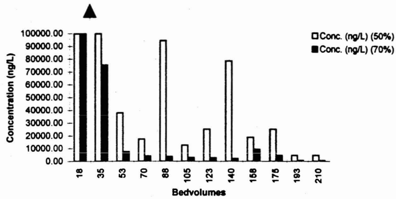
Figure 16: Comparison of Regeneration Cycles for EDB Removal (50 and 70% acetone). In first 35 bedvolumes treated, EDB concentrations exceed scale and reach 7 mg/L (indicated by arrow). Scale has been decreased in order to see lower concentrations.
