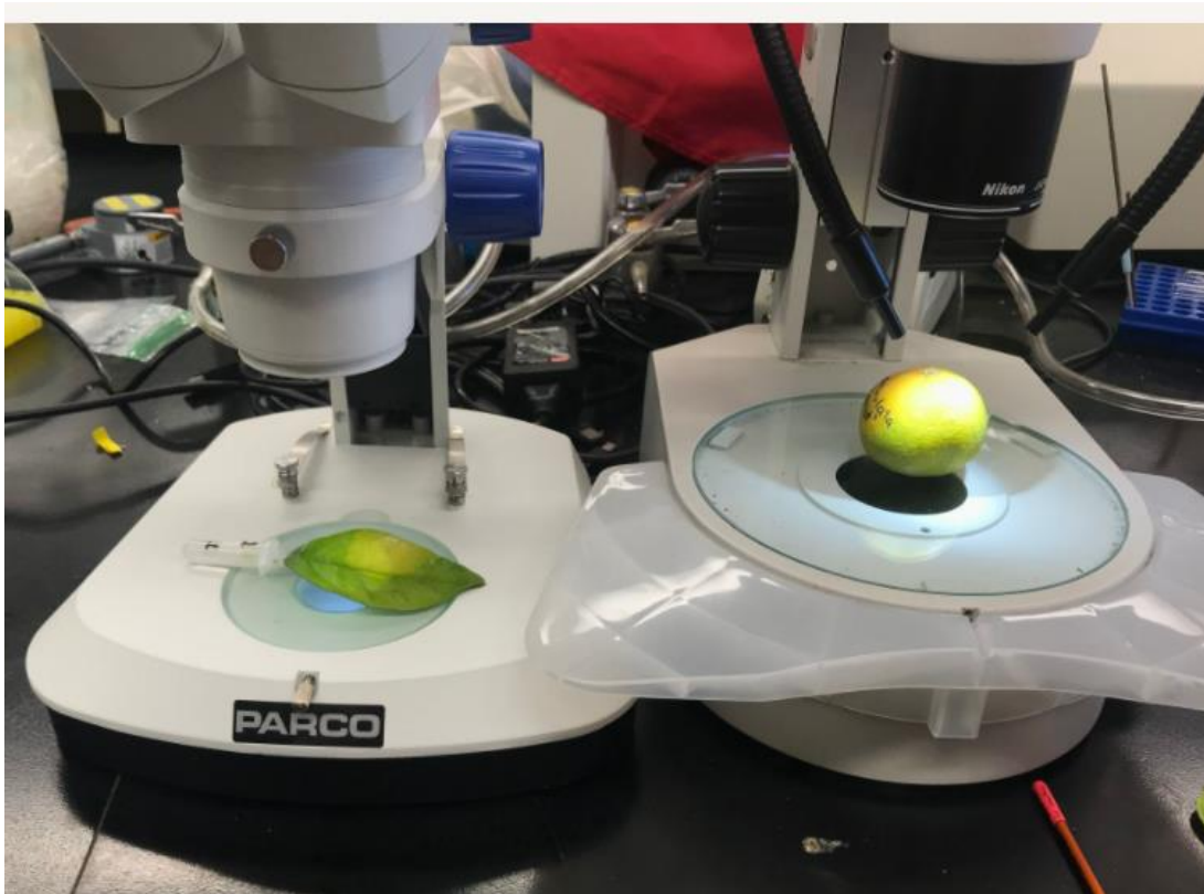
Figure 4.3 Set up for the transfer of Brevipalpus sp. mites from an isoline colony to a detached C. sinensis leaf presenting HGSV-2 symptoms and maintained in a 1.5 mL tube containing distilled water. Mite transfers and manipulations were performed using a number 01 fine Sable brush under a stereoscopic microscope.
